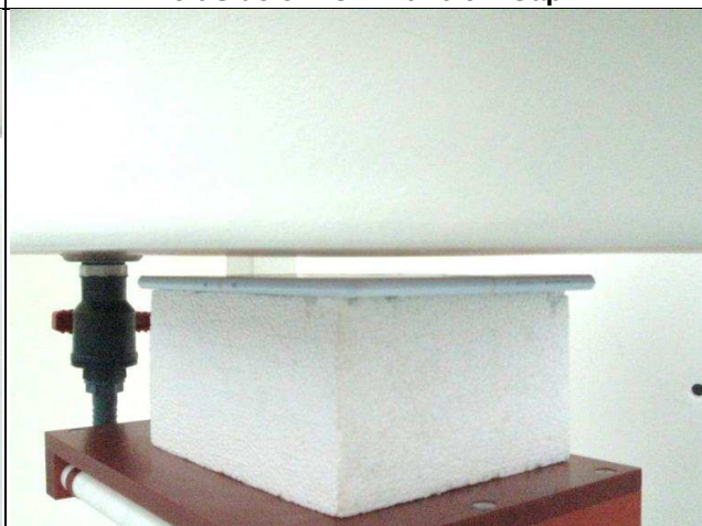
Rear Face of EUT with 1.0 cm Gap
