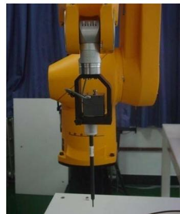
Picture C.3 E-field Probe
