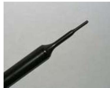
Picture C.2 Near-field Probe
