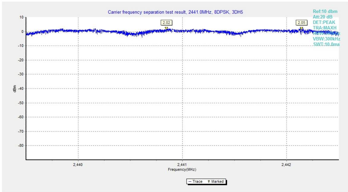
Fig.93. Carrier frequency separation measurement: 8DPSK, Channel 39
