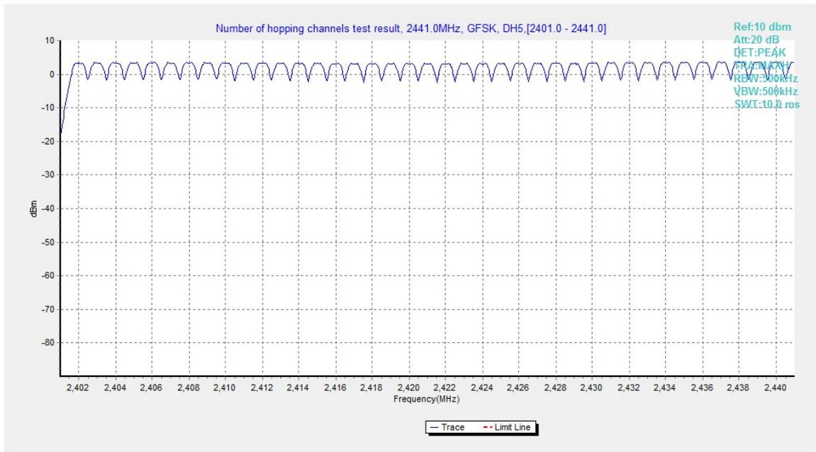
Fig.94. Number of hopping frequencies: GFSK, Channel 0 - 39
