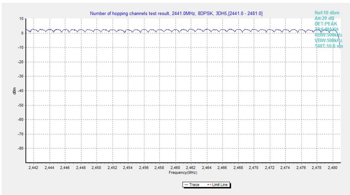
Fig.99. Number of hopping frequencies: 8DPSK, Channel 40 - 78
