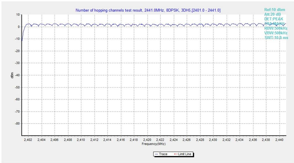
Fig.98. Number of hopping frequencies: 8DPSK, Channel 0 - 39
