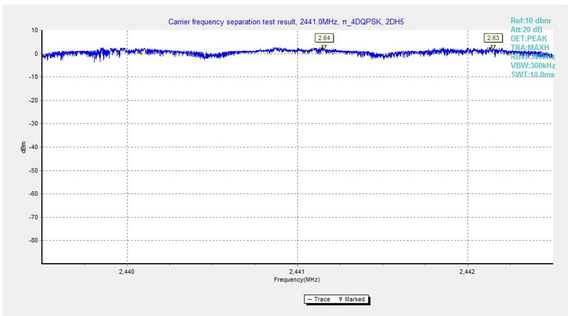
Fig.92. Carrier frequency separation measurement:  $\pi/4$  DQPSK, Channel 39
