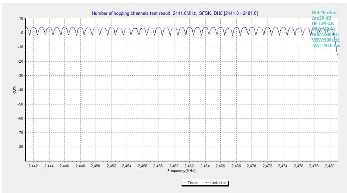
Fig.95. Number of hopping frequencies: GFSK, Channel 40 - 78
