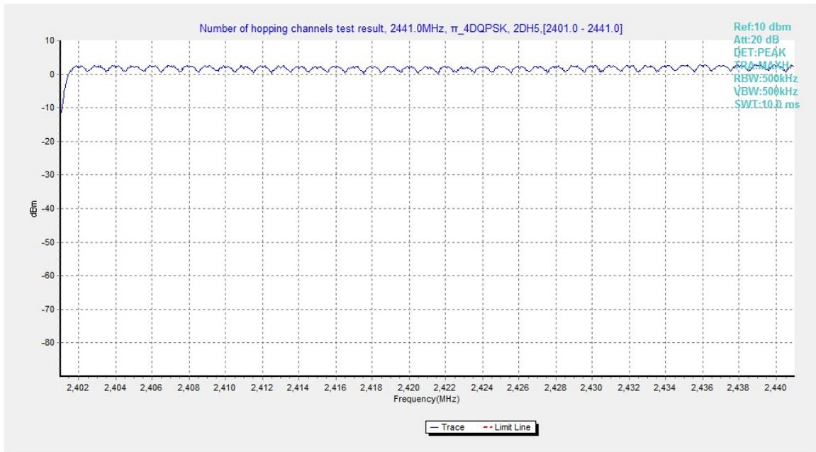
Fig.96. Number of hopping frequencies:  $\pi/4$  DQPSK, Channel 0 - 39
