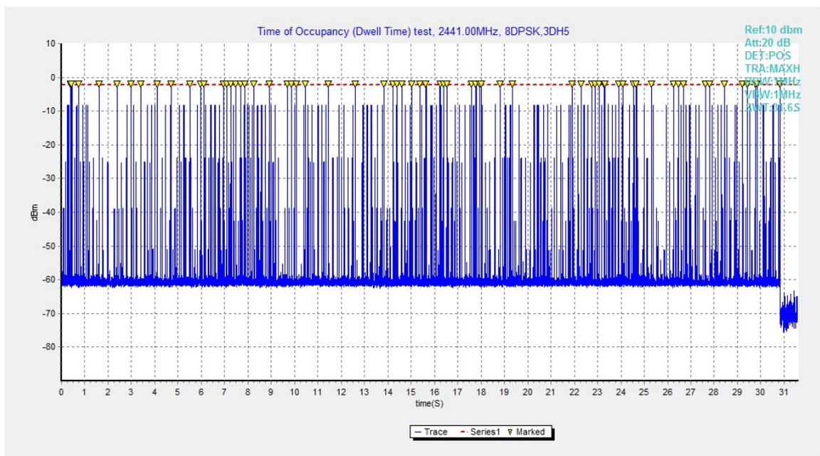
Fig.81. Number of Transmissions Measurement: Channel 39,Packet 3-DH5
