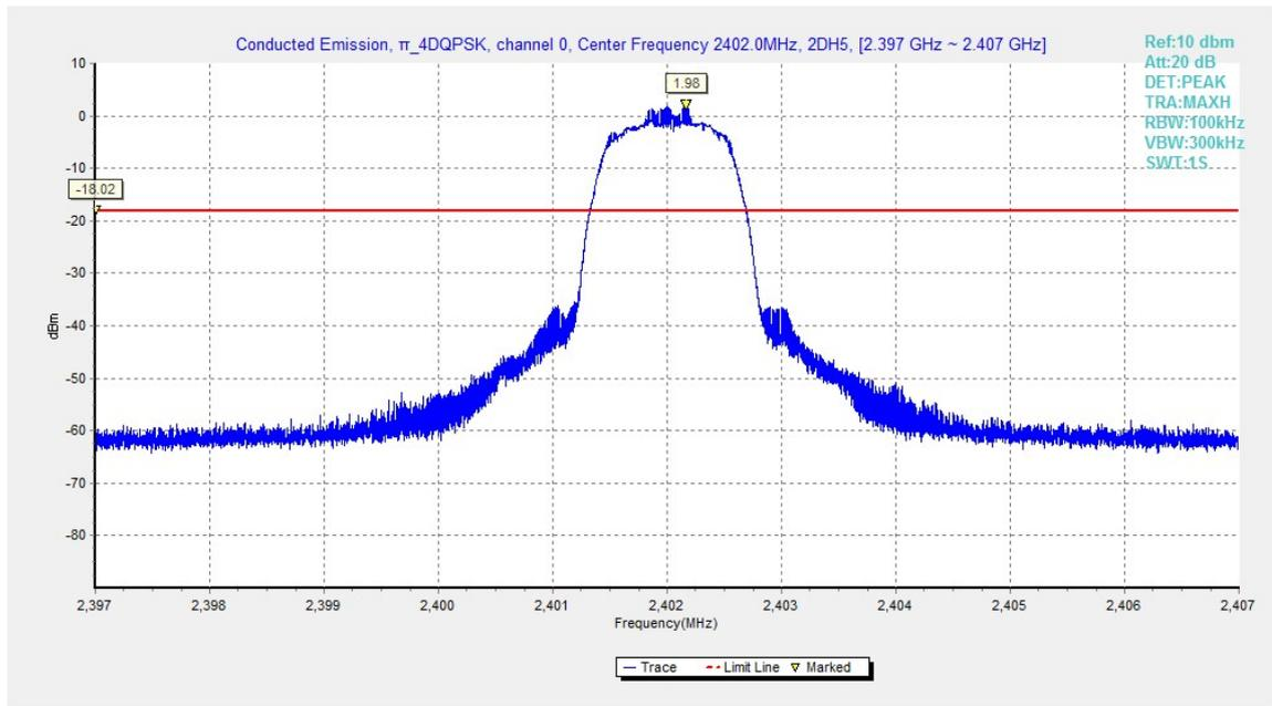
Fig.28. Conducted spurious emission:  $\pi/4$  DQPSK, Channel 0,2402MHz
