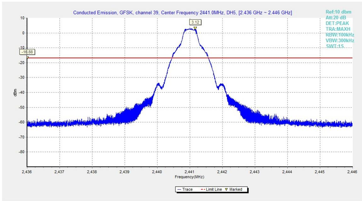
Fig.18. Conducted spurious emission: GFSK, Channel 39, 2441MHz
