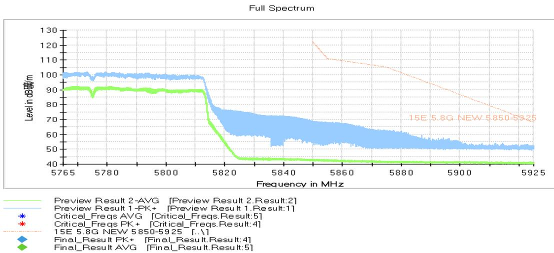
**Fig. 32 Band Edges (802.11ac-HT80, 5775MHz) BY EUT5**
