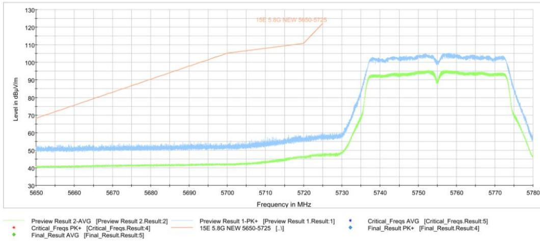
**Fig. 29 Band Edges (802.11n-HT40, 5755MHz) BY EUT5**
