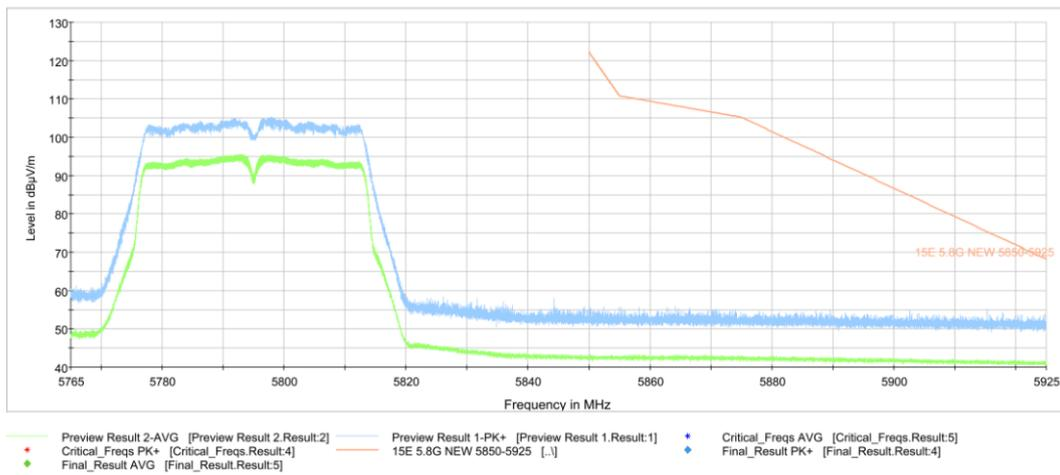
**Fig. 30 Band Edges (802.11n-HT40, 5795MHz) BY EUT5**
