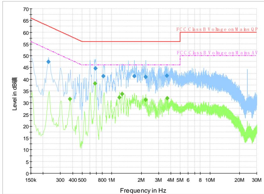
**Fig. 33 AC Powerline Conducted Emission-802.11a**
