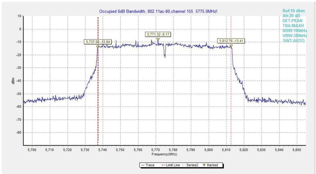
**Fig. 14 Occupied 6dB Bandwidth (802.11ac-HT80, Ch 155)**
