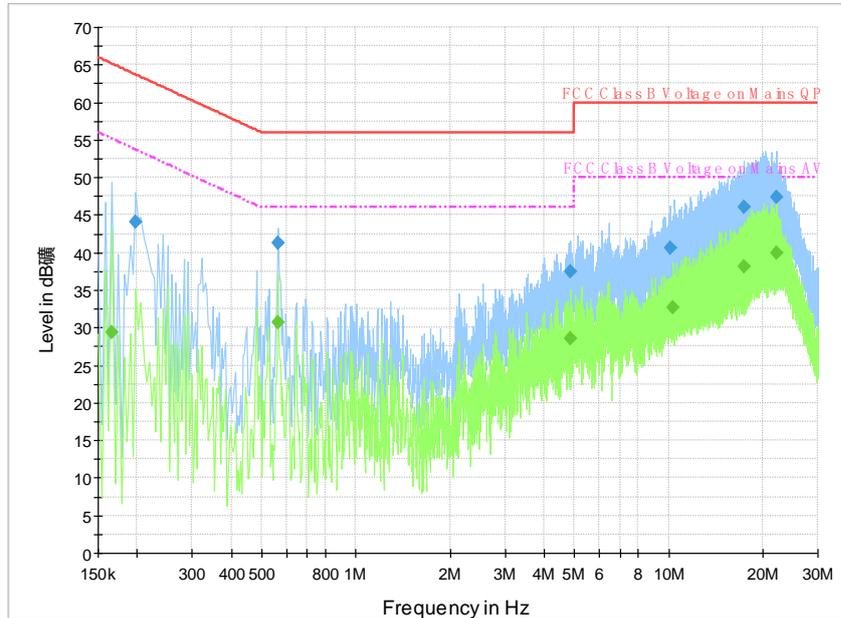
Fig. 35 AC Powerline Conducted Emission-802.11a
