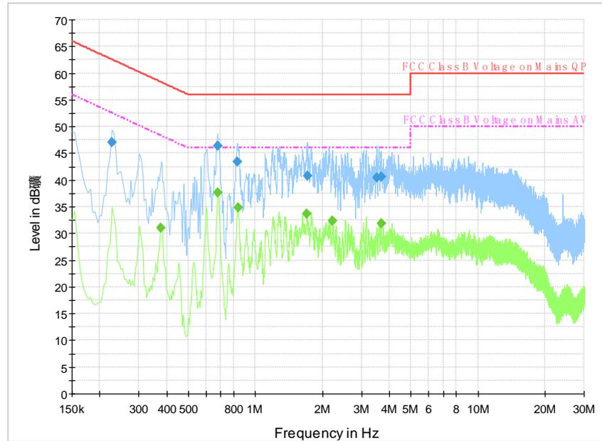
Fig. 34 AC Powerline Conducted Emission-Idle
