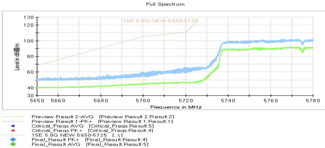
**Fig. 31 Band Edges (802.11ac-HT80, 5775MHz) BY EUT5**
