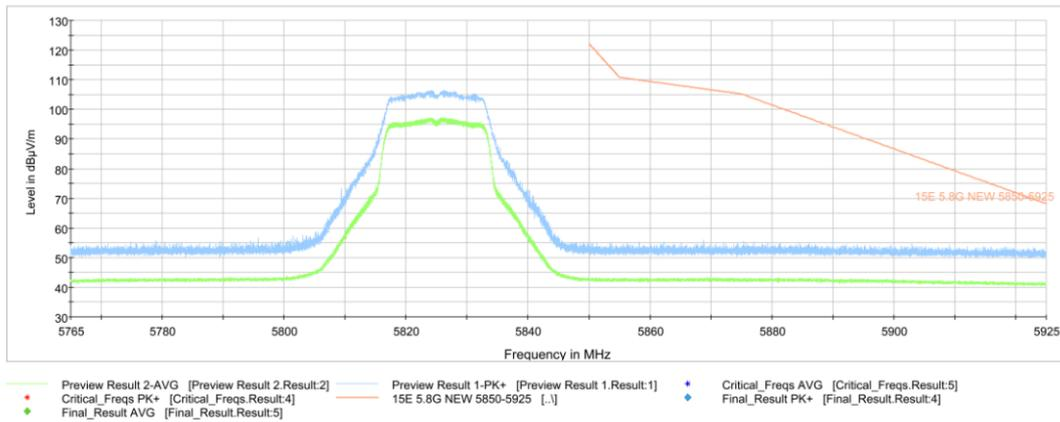
**Fig. 28 Band Edges (802.11a, 5825MHz) BY EUT5**
