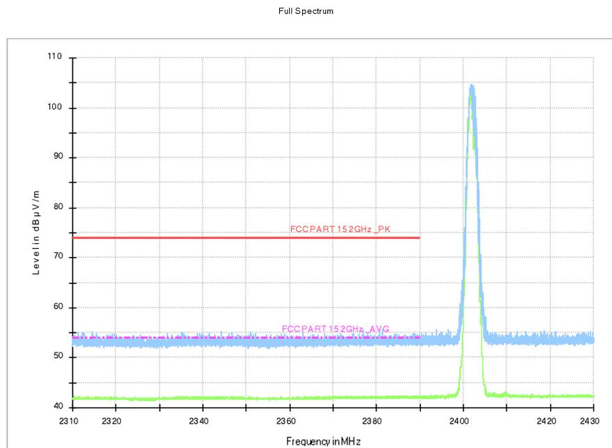
Fig.3. Frequency Band Edges: GFSK, 2402 MHz, 2.31 GHz – 2.45GHz
