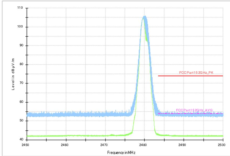
**Fig.4. Frequency Band Edges: GFSK, 2480 MHz, 2.45 GHz - 2.50GHz**
