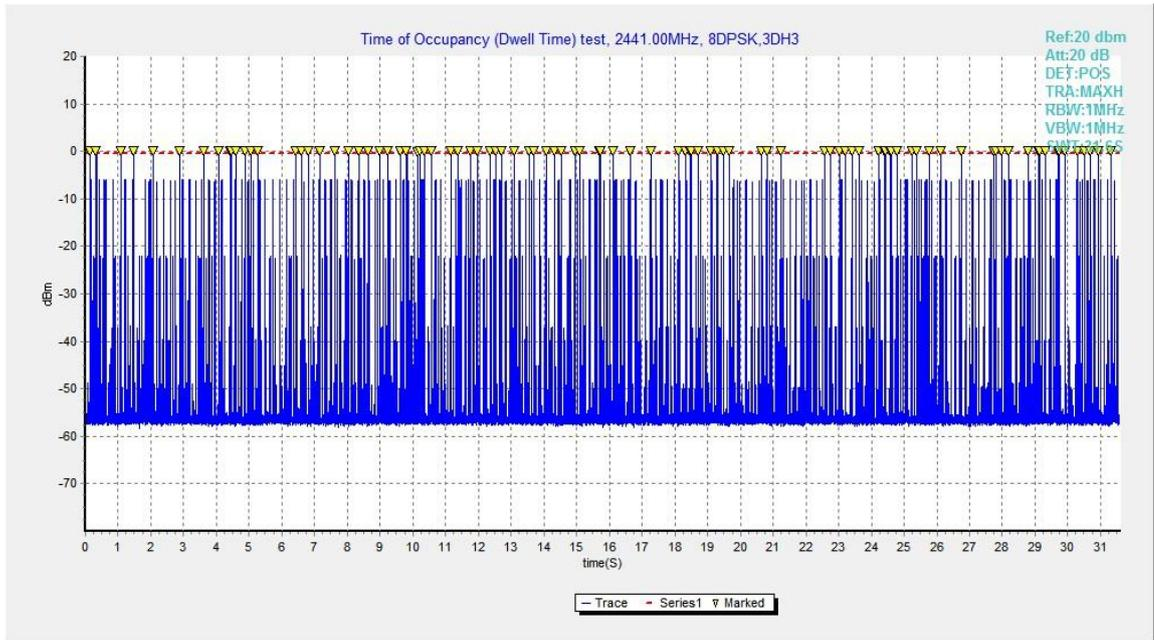
Fig.79. Number of Transmissions Measurement: Channel 39,Packet 3-DH3
