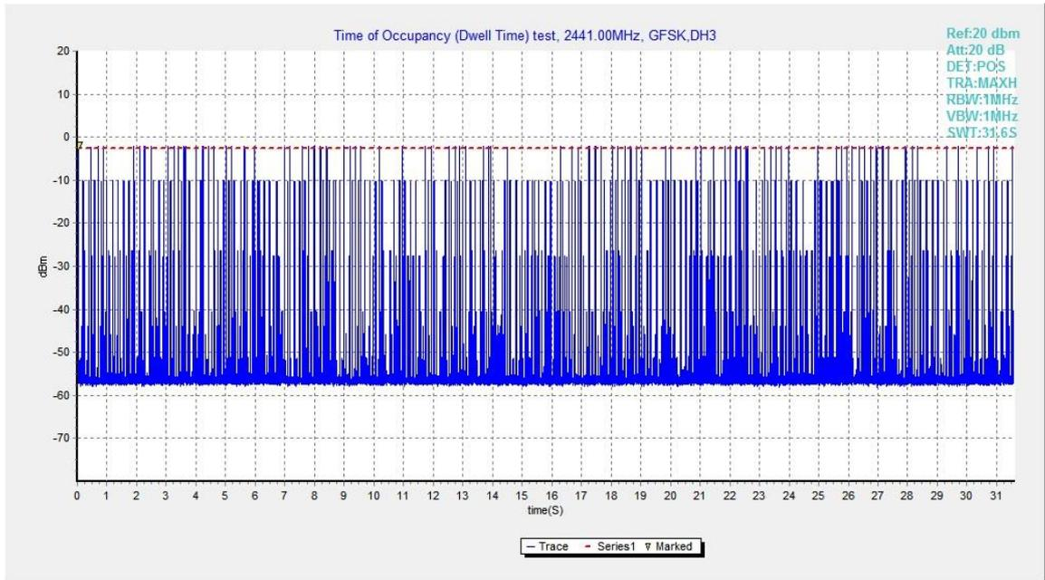
Fig.67. Number of Transmissions Measurement: Channel 39,Packet DH3
