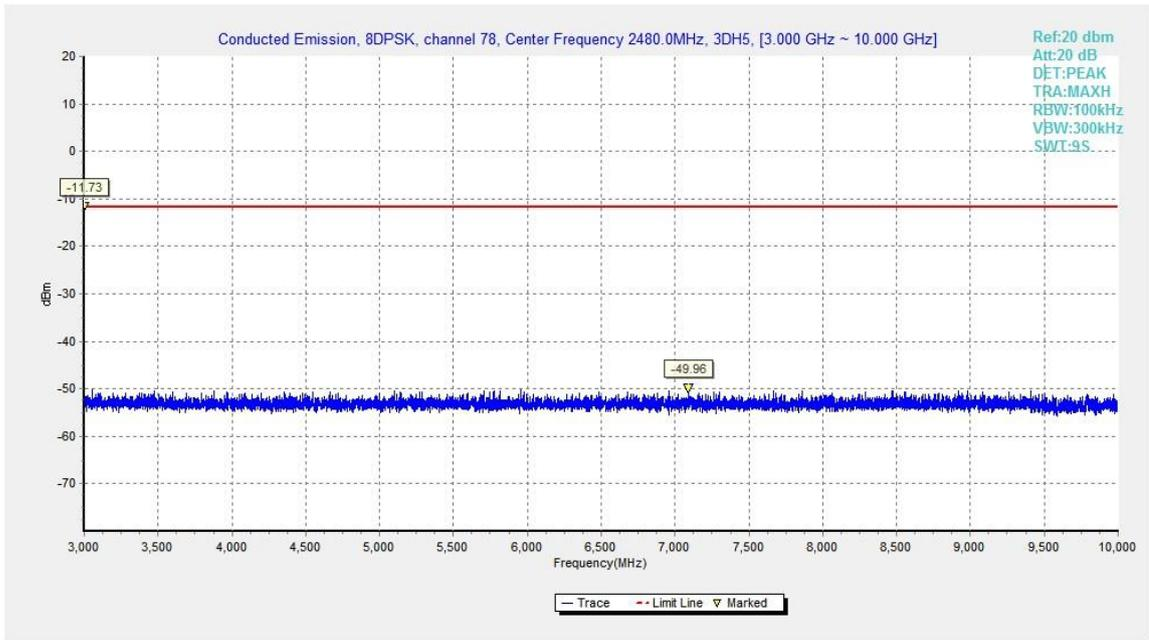
Fig.62. Conducted spurious emission: 8DPSK, Channel 78, 3GHz - 10GHz
