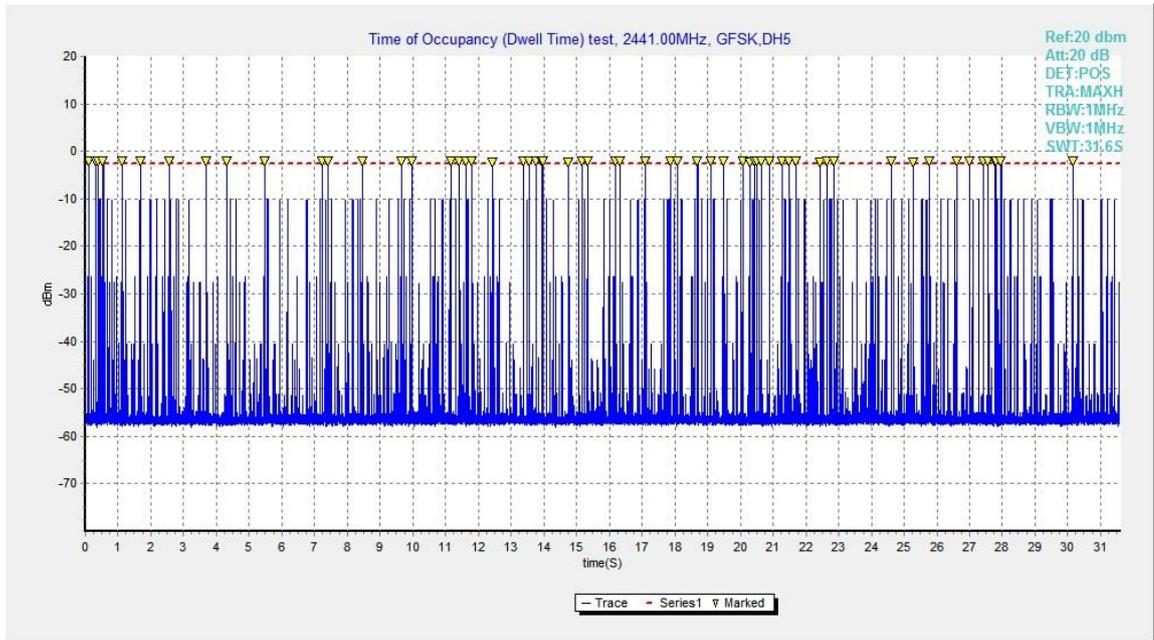
Fig.69. Number of Transmissions Measurement: Channel 39,Packet DH5
