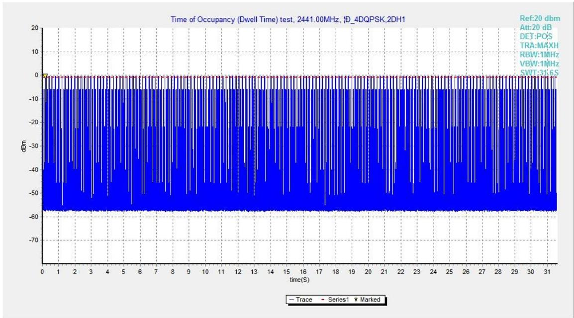
Fig.71. Number of Transmissions Measurement: Channel 39,Packet 2-DH1
