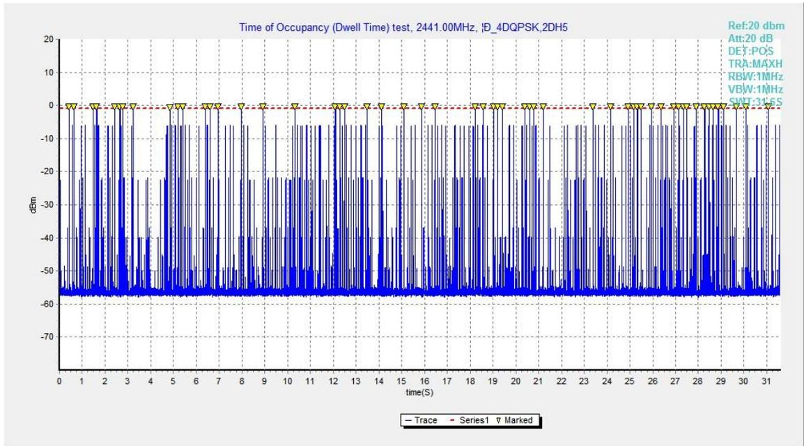
Fig.75. Number of Transmissions Measurement: Channel 39,Packet 2-DH5
