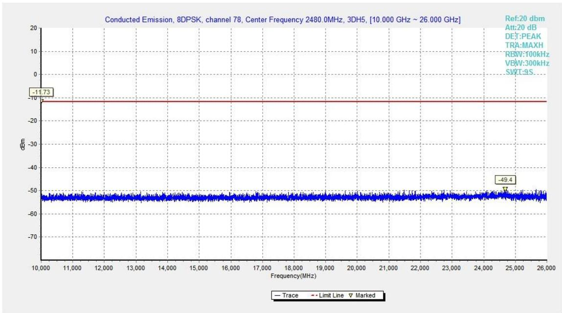
Fig.63. Conducted spurious emission: 8DPSK, Channel 78, 10GHz - 26GHz
