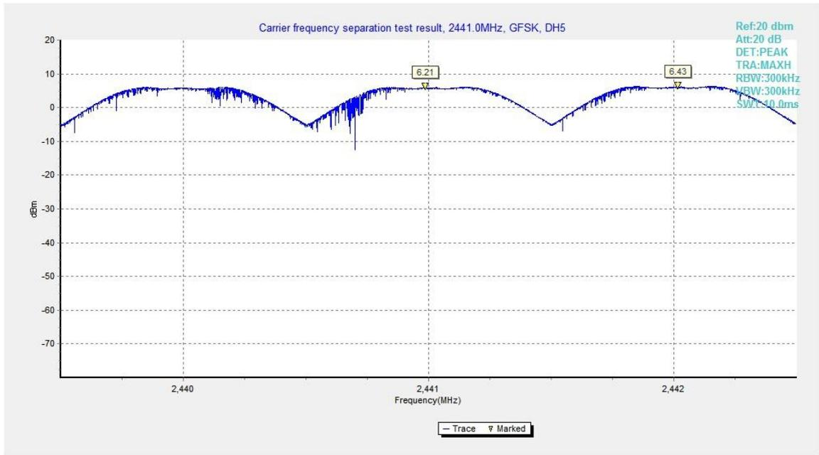
Fig.91. Carrier frequency separation measurement: GFSK, Channel 39
