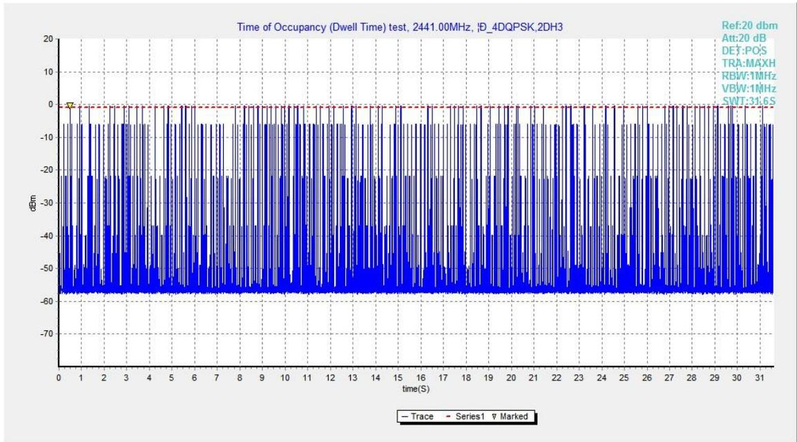
Fig.73. Number of Transmissions Measurement: Channel 39,Packet 2-DH3
