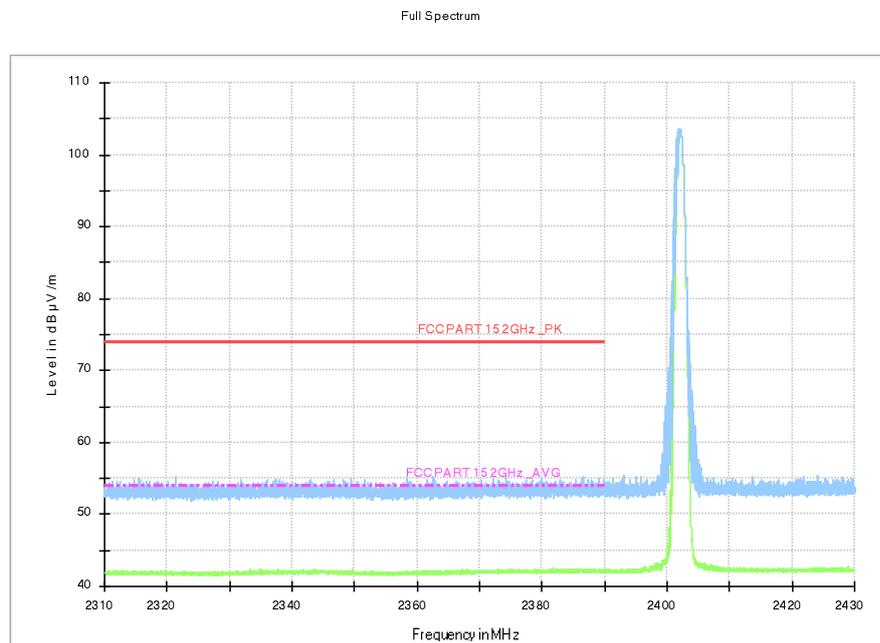
Fig.13. Frequency Band Edges: GFSK, Channel 0, 2.31 GHz – 2.45GHz
