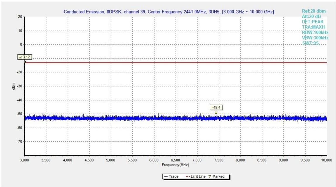
Fig.57. Conducted spurious emission: 8DPSK, Channel 39, 3GHz - 10GHz
