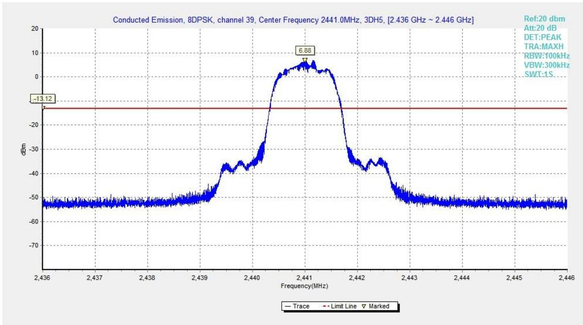
Fig.54. Conducted spurious emission: 8DPSK, Channel 39, 2441MHz
