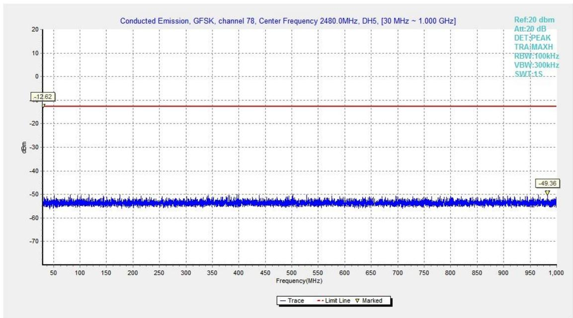
Fig.30. Conducted spurious emission: GFSK, Channel 78, 30MHz - 1GHz
