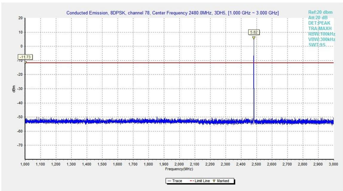
Fig.61. Conducted spurious emission: 8DPSK, Channel 78, 1GHz - 3GHz
