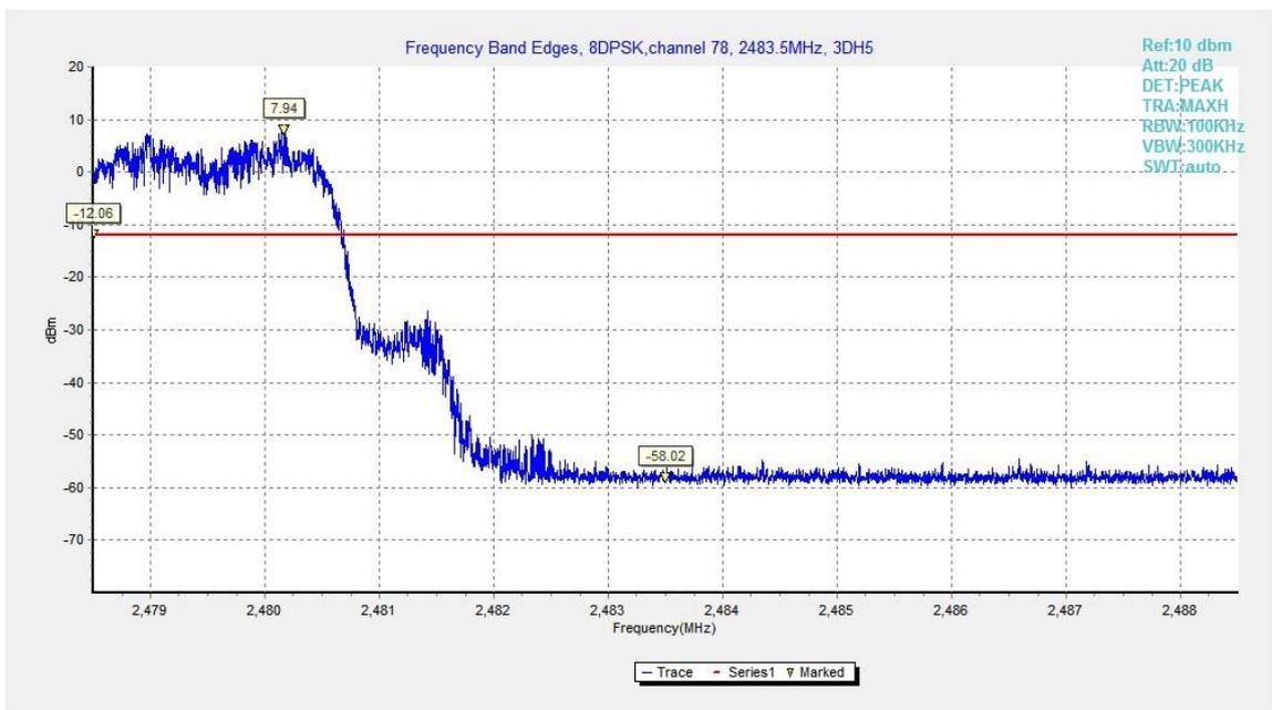
Fig.12. Frequency Band Edges: 8DPSK, Channel 78, Hopping On
