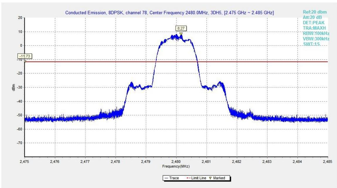
Fig.59. Conducted spurious emission: 8DPSK, Channel 78, 2480MHz
