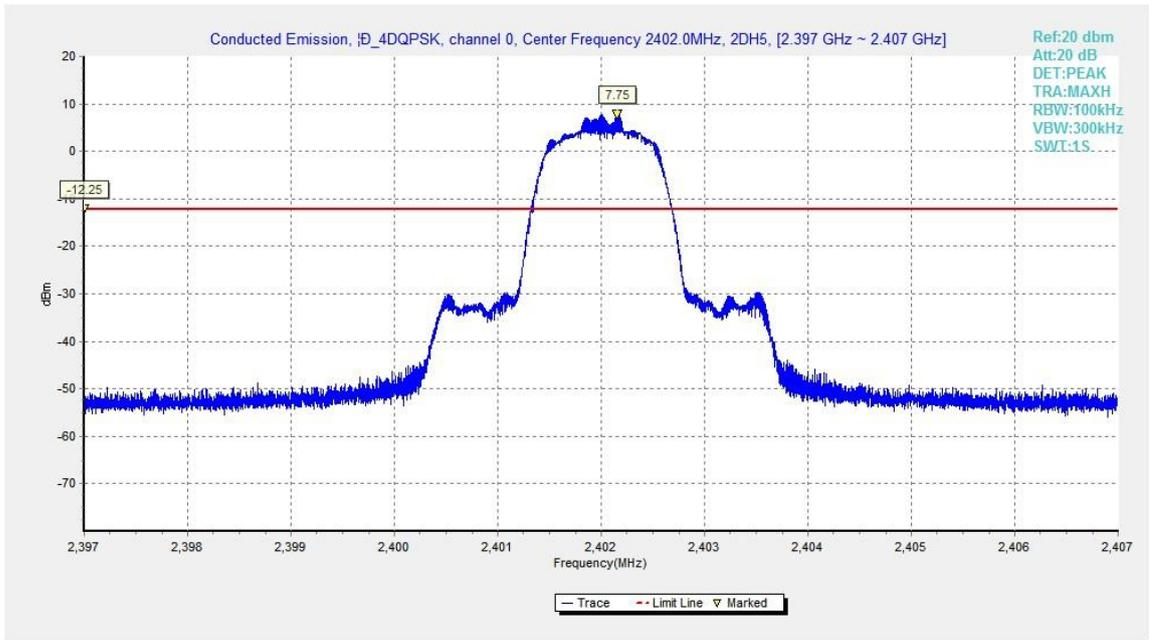
Fig.34. Conducted spurious emission:  $\pi/4$  DQPSK, Channel 0,2402MHz
