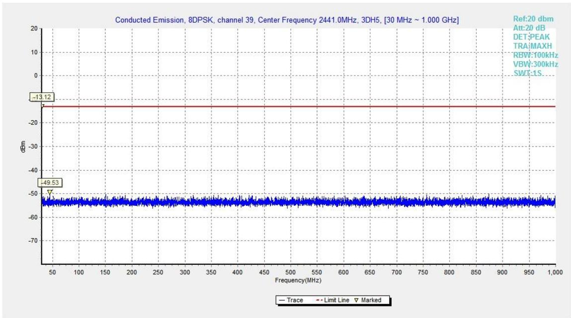
Fig.55. Conducted spurious emission: 8DPSK, Channel 39, 30MHz - 1GHz
