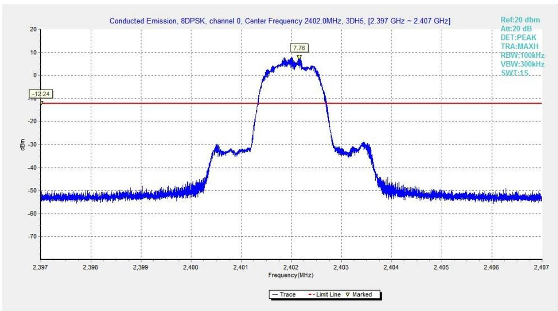
Fig.49. Conducted spurious emission: 8DPSK, Channel 0, 2,402MHz
