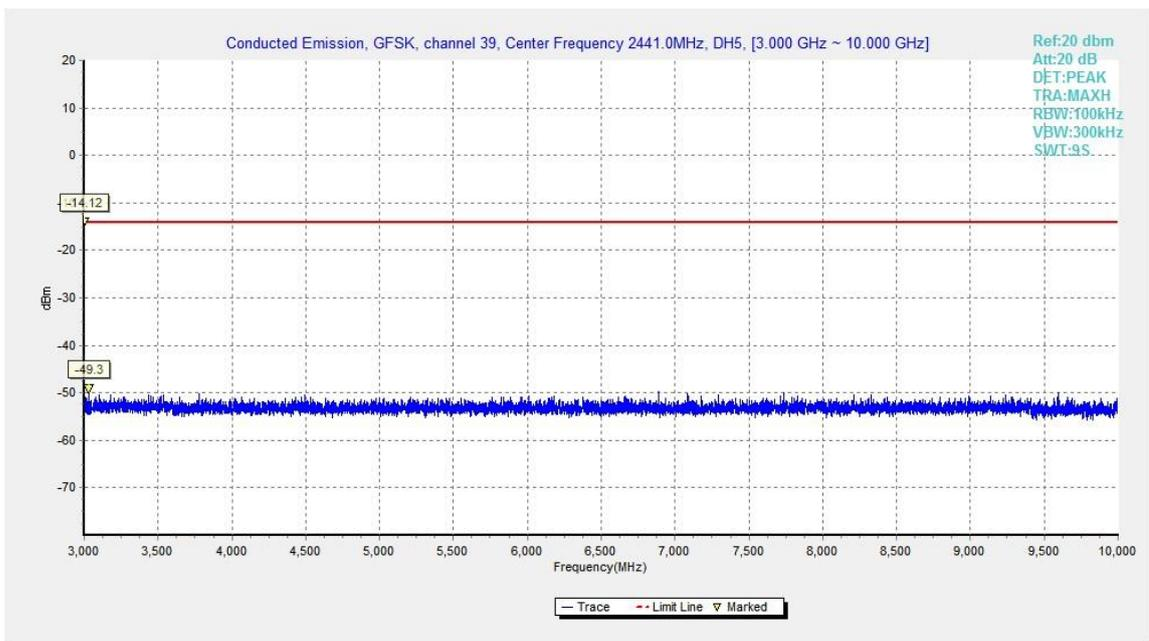
Fig.27. Conducted spurious emission: GFSK, Channel 39, 3GHz – 10GHz
