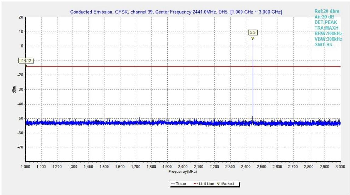
Fig.26. Conducted spurious emission: GFSK, Channel 39, 1GHz – 3GHz
