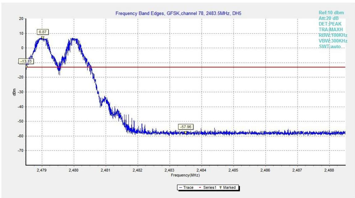
Fig.4. Frequency Band Edges: GFSK, Channel 78, Hopping On
