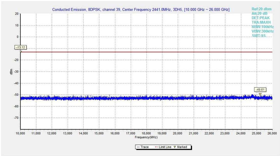
Fig.58. Conducted spurious emission: 8DPSK, Channel 39, 10GHz – 26GHz
