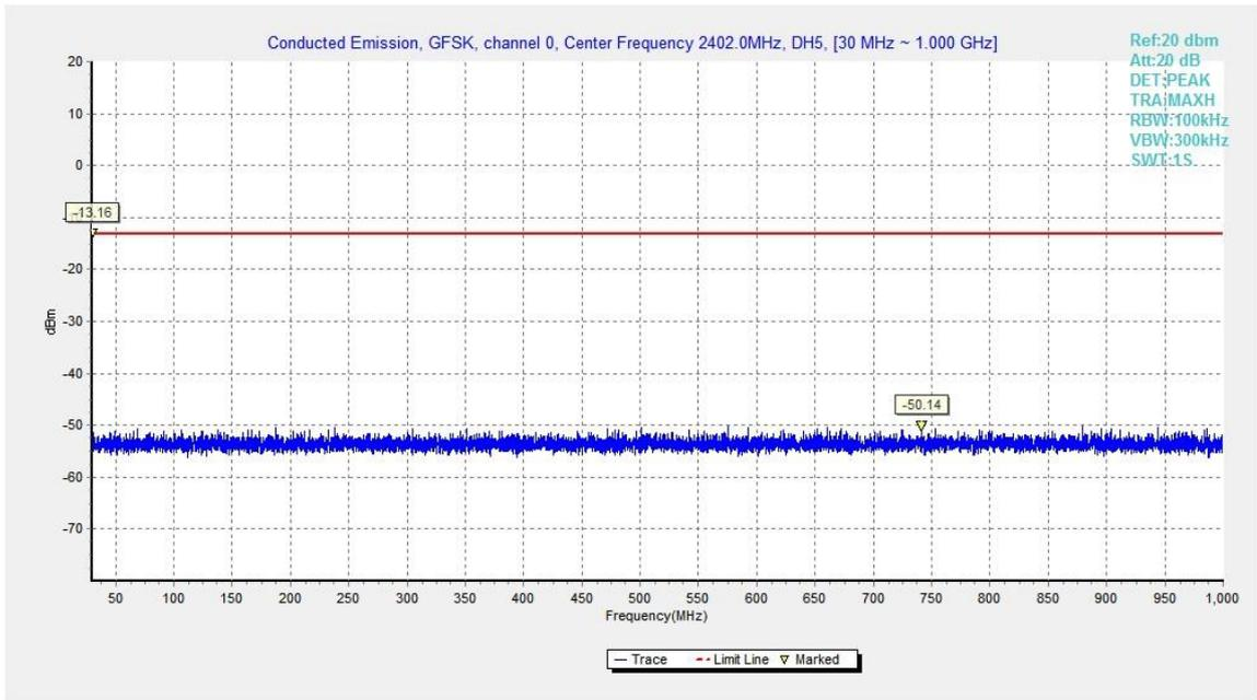
Fig.20. Conducted spurious emission: GFSK, Channel 0, 30MHz - 1GHz
