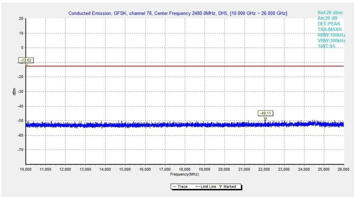
Fig.33. Conducted spurious emission: GFSK, Channel 78, 10GHz - 26GHz
