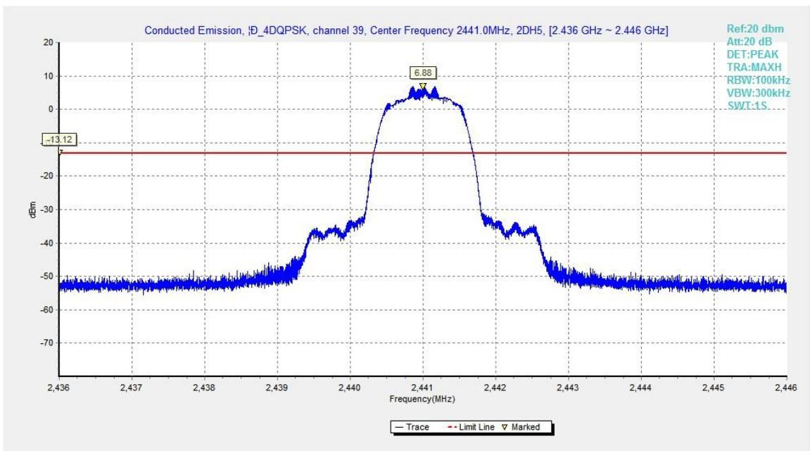
Fig.39. Conducted spurious emission:  $\pi/4$  DQPSK, Channel 39, 2441MHz
