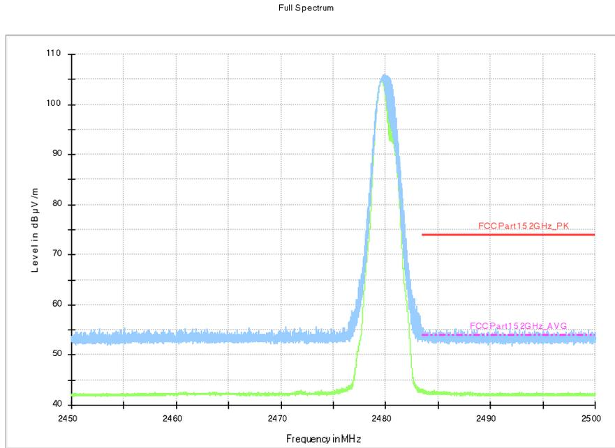
**Fig.18. Frequency Band Edges: 8DPSK, Channel 78, 2.45 GHz - 2.50GHz**
