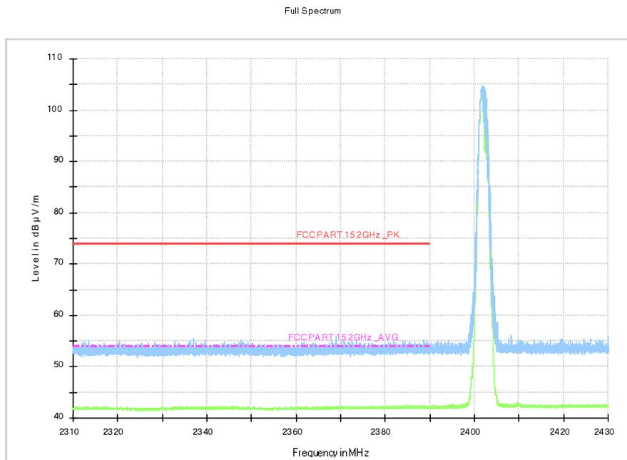
**Fig.17. Frequency Band Edges: 8DPSK, Channel 0, 2.38 GHz - 2.45GHz**
