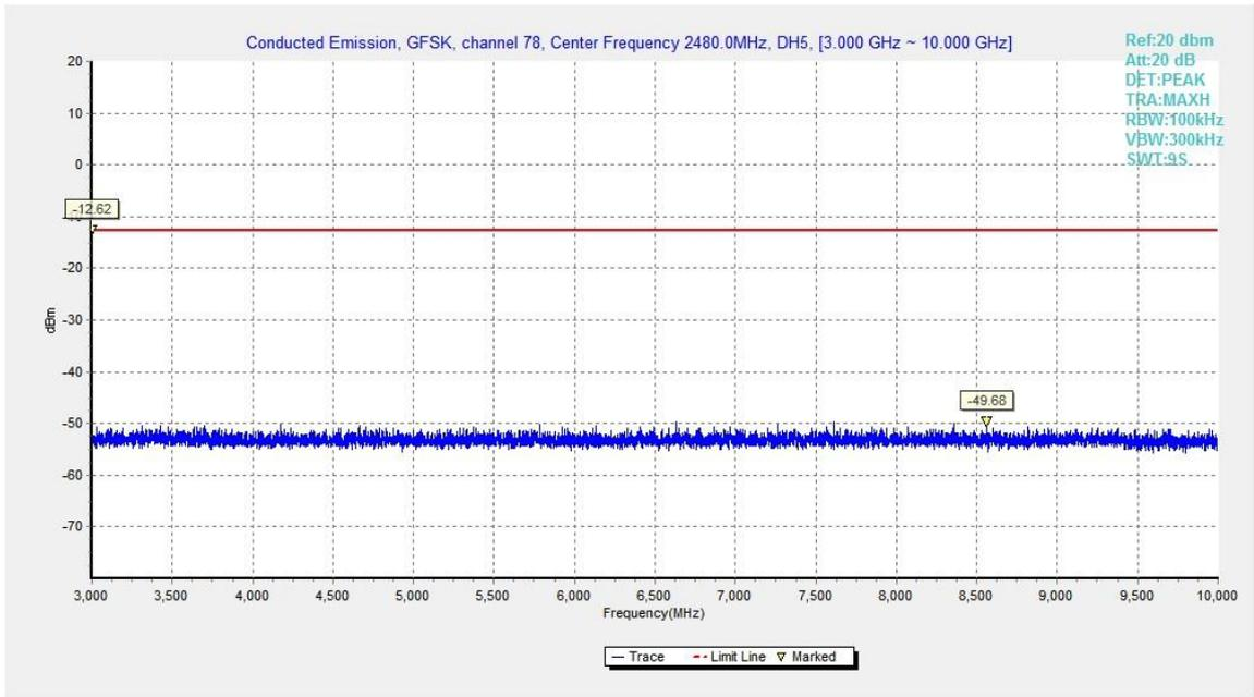
Fig.32. Conducted spurious emission: GFSK, Channel 78, 3GHz - 10GHz
