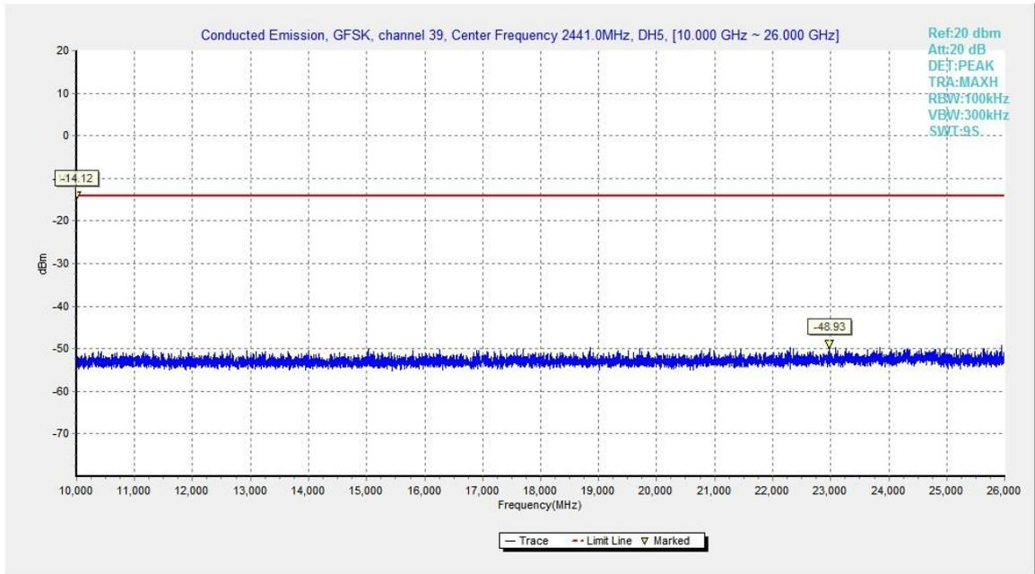
Fig.28. Conducted spurious emission: GFSK, Channel 39, 10GHz – 26GHz
