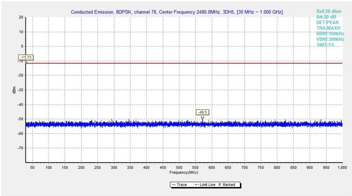
Fig.60. Conducted spurious emission: 8DPSK, Channel 78, 30MHz - 1GHz
