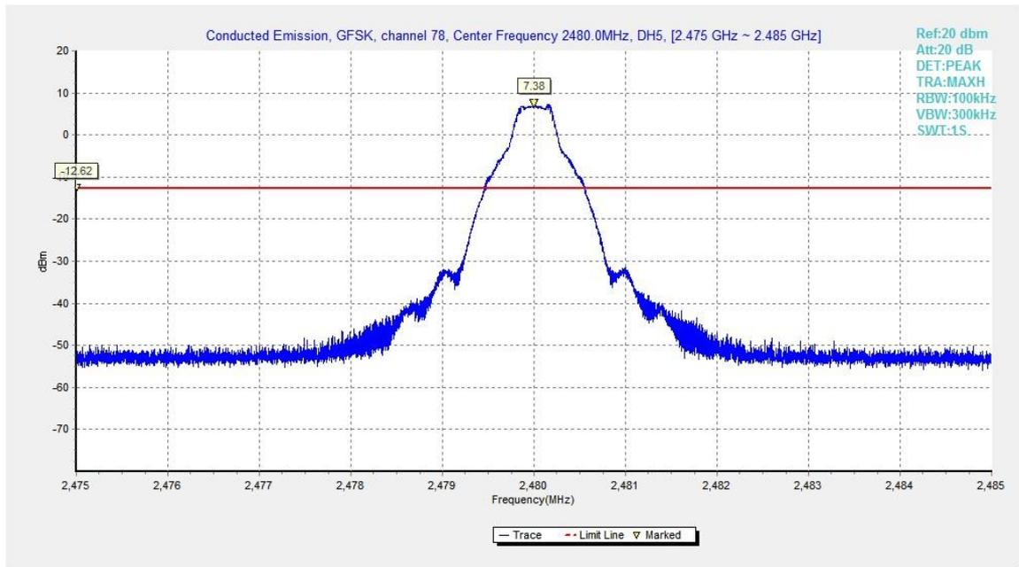
Fig.29. Conducted spurious emission: GFSK, Channel 78, 2480MHz
