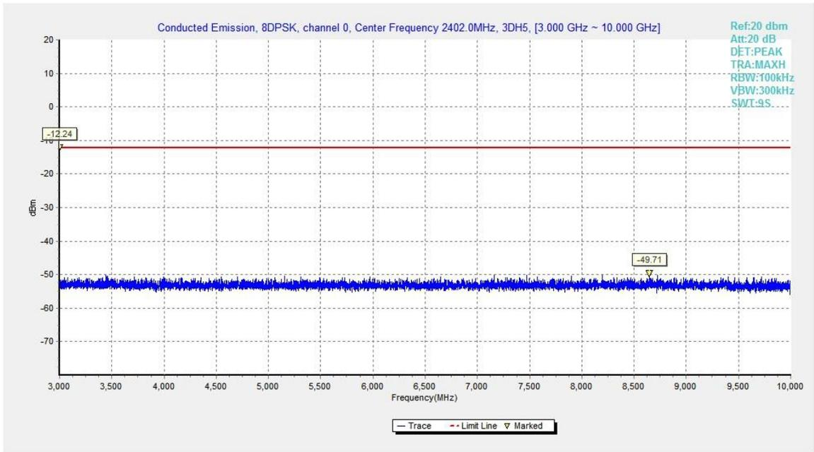
Fig.52. Conducted spurious emission: 8DPSK, Channel 0, 3GHz - 10GHz
