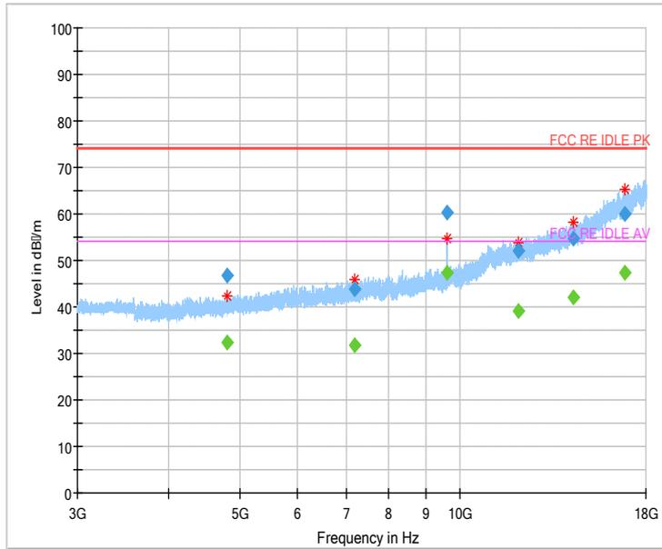
Fig.47 Radiated emission:  $\pi/4$  DQPSK, Ch0, 3GHz~18GHz
