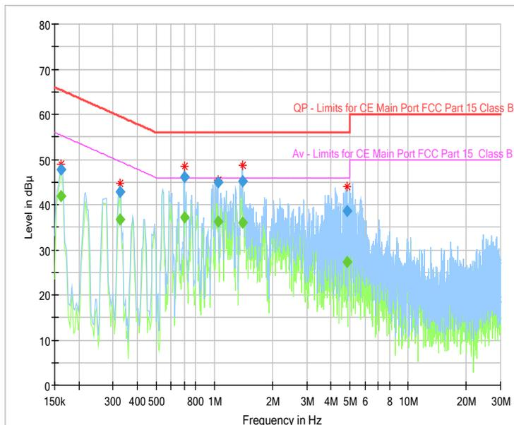
**Fig.91 AC Powerline Conducted Emission**
