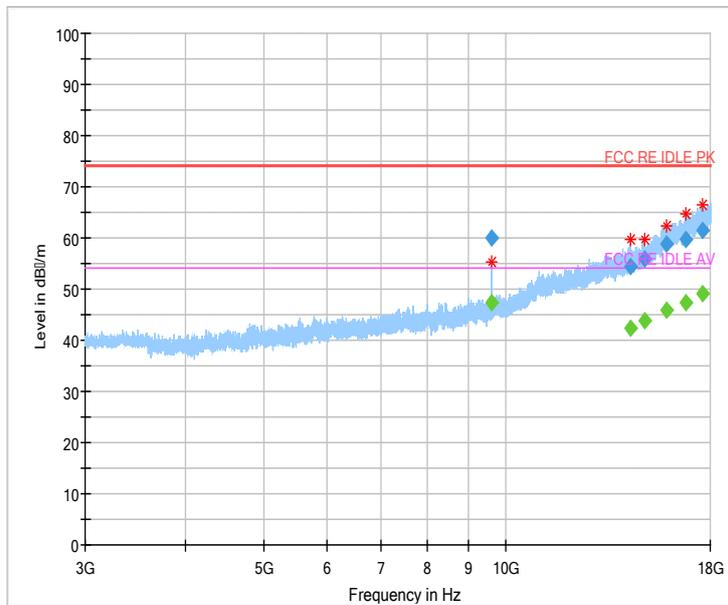
Fig.52 Radiated emission: 8DPSK, Ch0, 3GHz~18GHz
