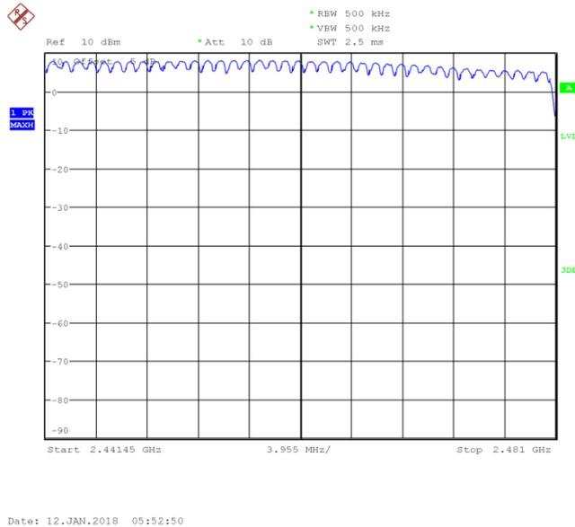
Fig.90 Number of hopping frequency: 8DPSK, Ch40~78
