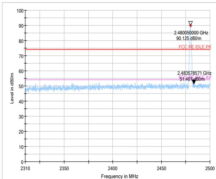
Fig.54 Radiated emission (Power): 8DPSK, high channel
