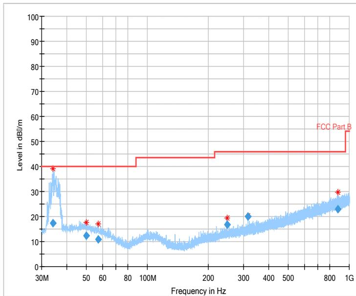
Fig.50 Radiated emission: 8DPSK, Ch0, 30MHz~1GHz
