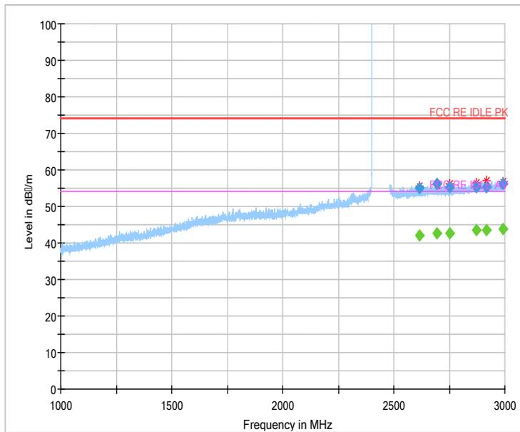
Fig.46 Radiated emission:  $\pi/4$  DQPSK, Ch0, 1GHz~3GHz
