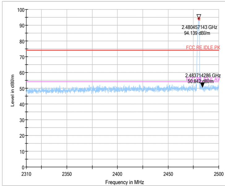
Fig.49 Radiated emission (Power):  $\pi/4$  DQPSK, high channel
