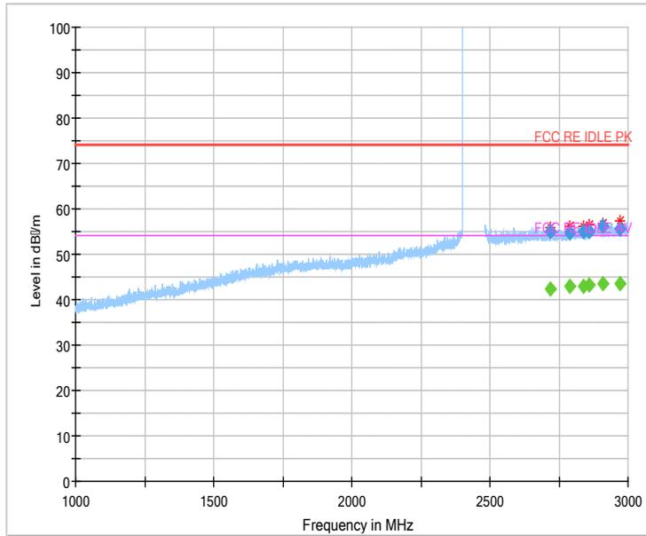
Fig.51 Radiated emission: 8DPSK, Ch0, 1GHz~3GHz
