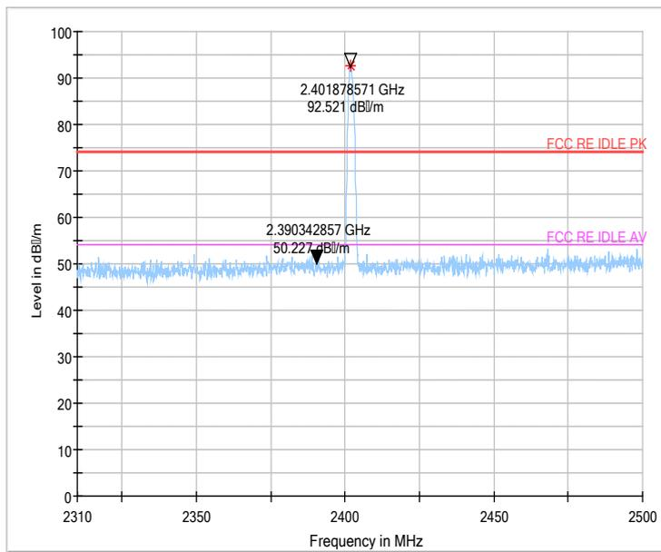
Fig.53 Radiated emission (Power): 8DPSK, low channel
