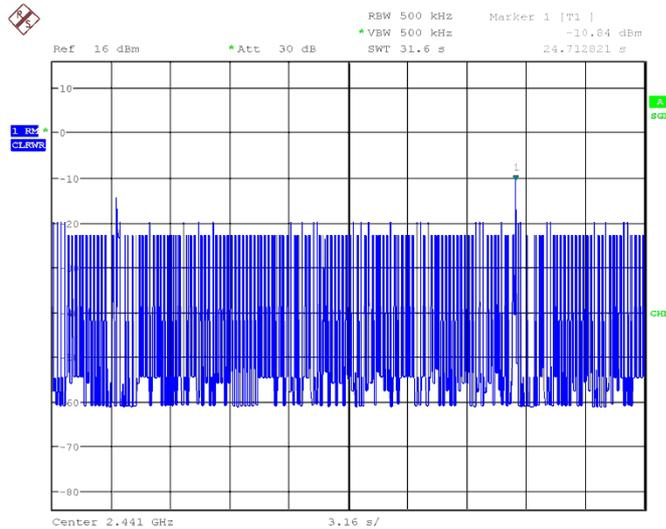
Fig.62 Number of Transmissions Measurement: Ch39, Packet 2-DH1
