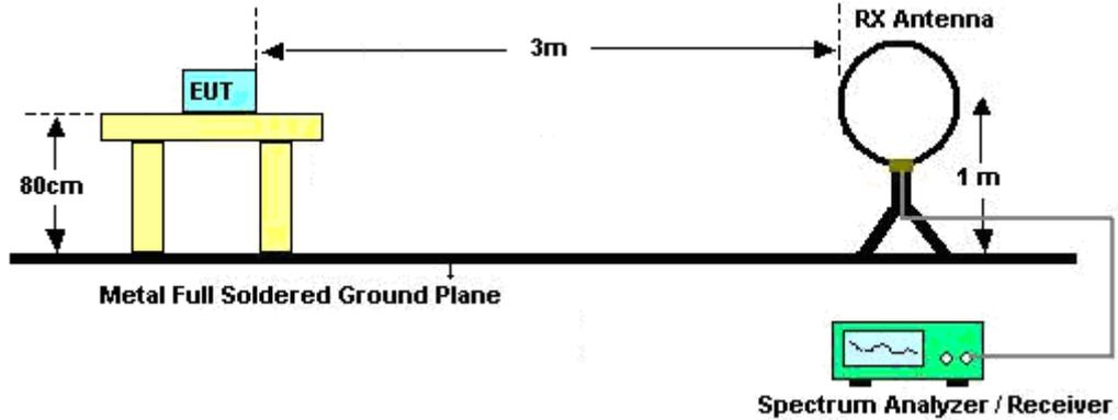
For radiated emissions from 30MHz to 1GHz
