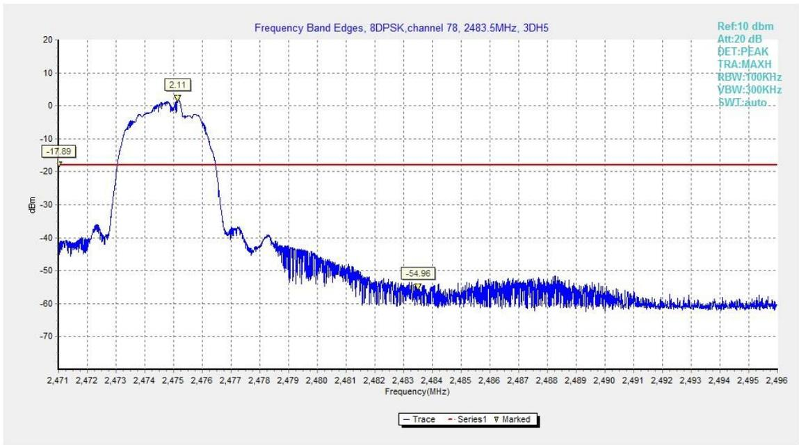
Fig.11. Frequency Band Edges: 8DPSK, Channel 78, Hopping Off
