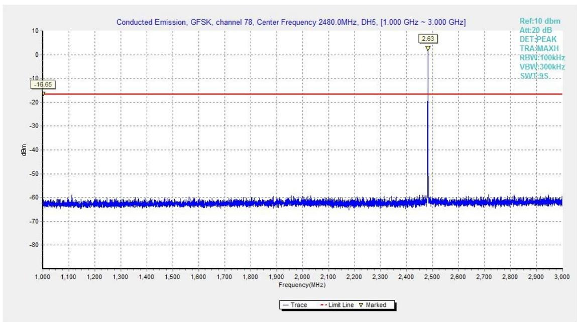
Fig.25. Conducted spurious emission: GFSK, Channel 78, 1GHz - 3GHz
