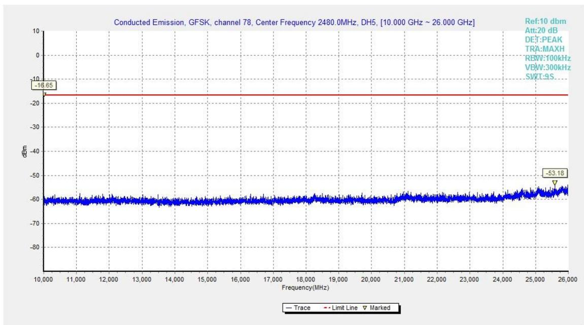
Fig.27. Conducted spurious emission: GFSK, Channel 78, 10GHz - 26GHz
