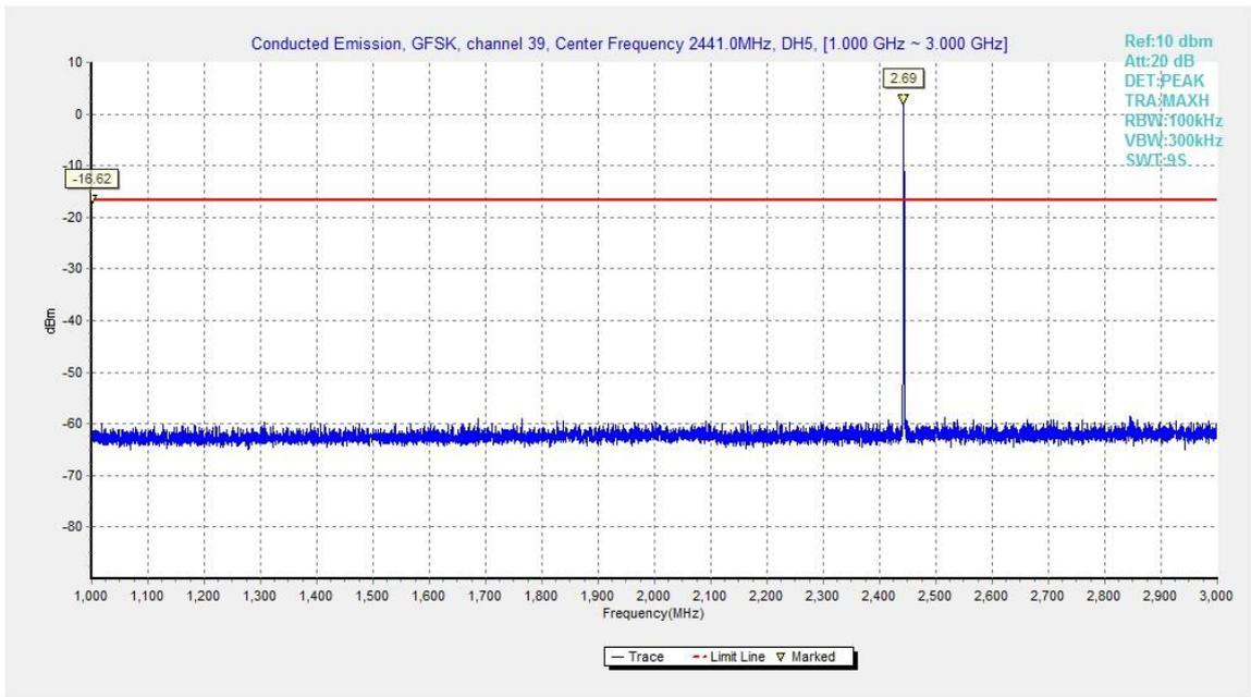
Fig.20. Conducted spurious emission: GFSK, Channel 39, 1GHz – 3GHz
