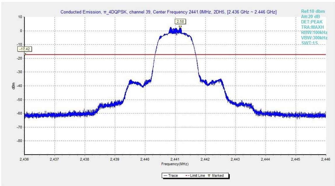
Fig.33. Conducted spurious emission:  $\pi/4$  DQPSK, Channel 39, 2441MHz
