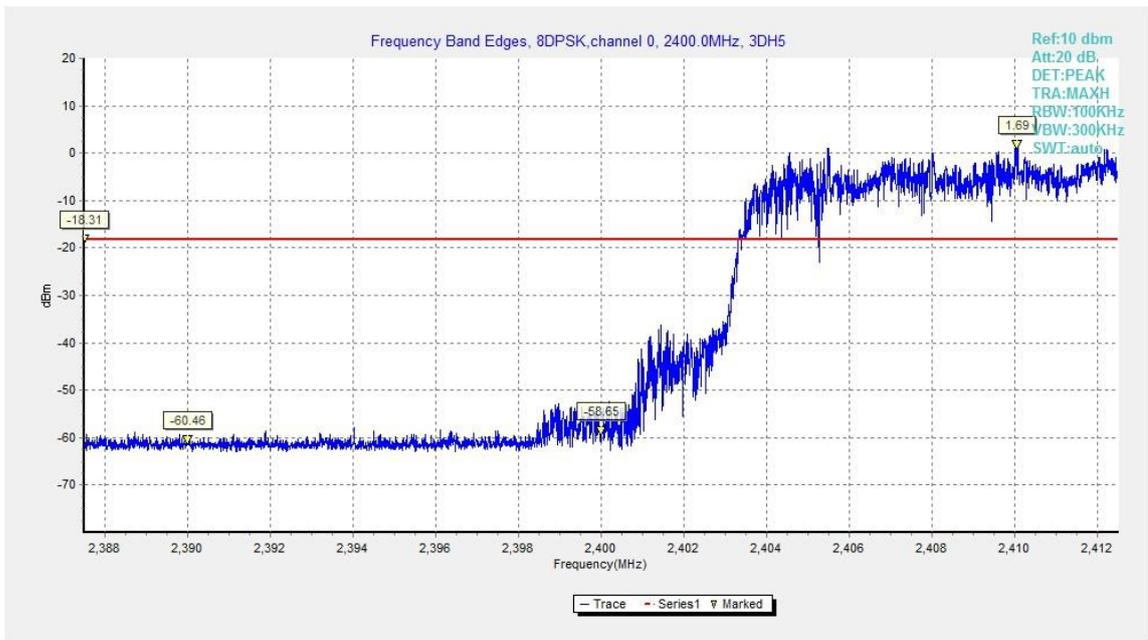
Fig.10. Frequency Band Edges: 8DPSK, Channel 0, Hopping On
