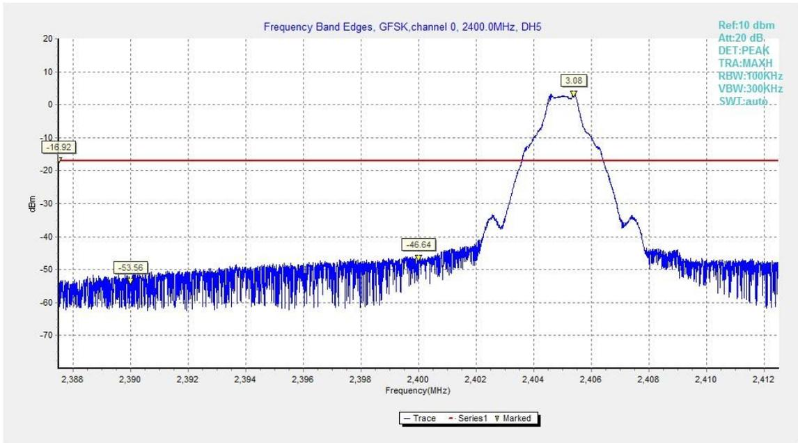
Fig.1. Frequency Band Edges: GFSK, Channel 0, Hopping Off
