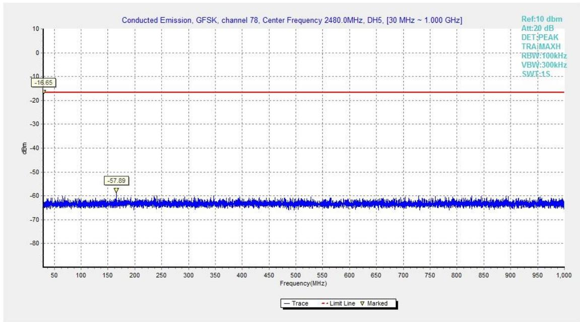
Fig.24. Conducted spurious emission: GFSK, Channel 78, 30MHz - 1GHz
