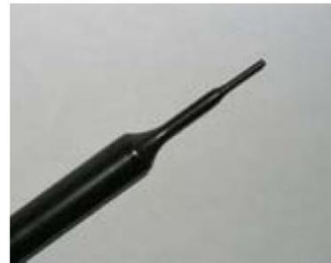
Picture C.2 Near-field Probe
