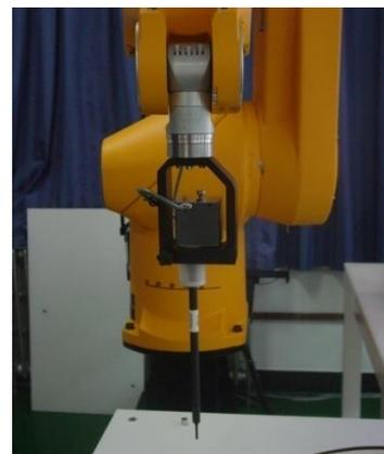
Picture C.3 E-field Probe
