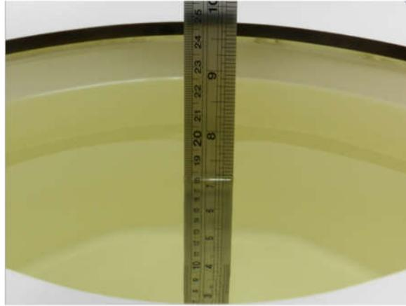
**Fig 11.1 Photo of Liquid Height for Body SAR**
