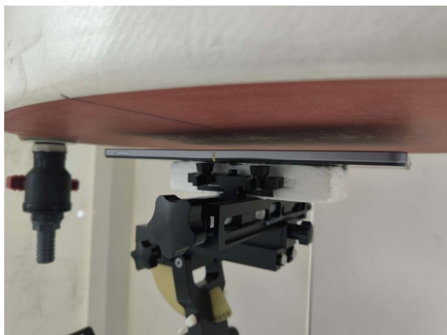
Bottom Face, Test Separation 20 mm
