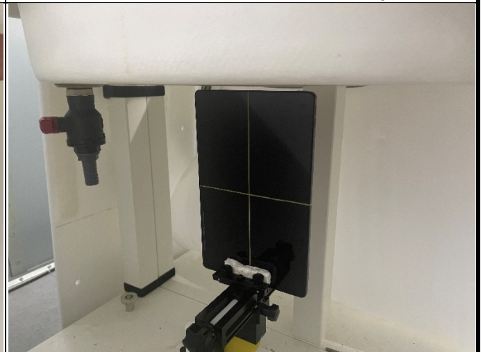
Left Side of EUT with 0.5 cm Gap
