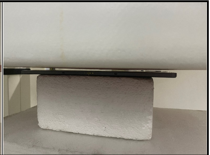
Rear Face of EUT with 0.5 cm Gap
