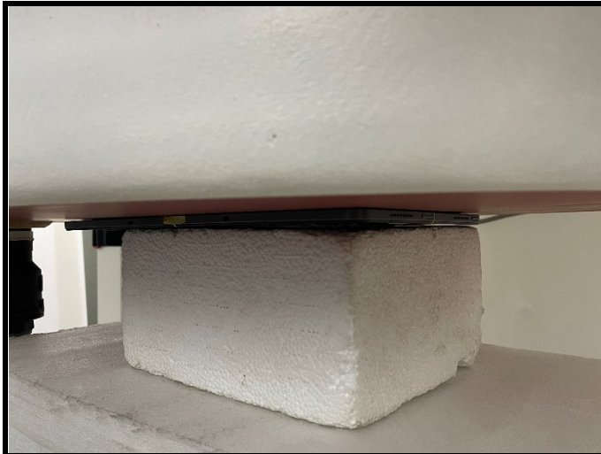
Rear Face of EUT with 0 cm Gap
