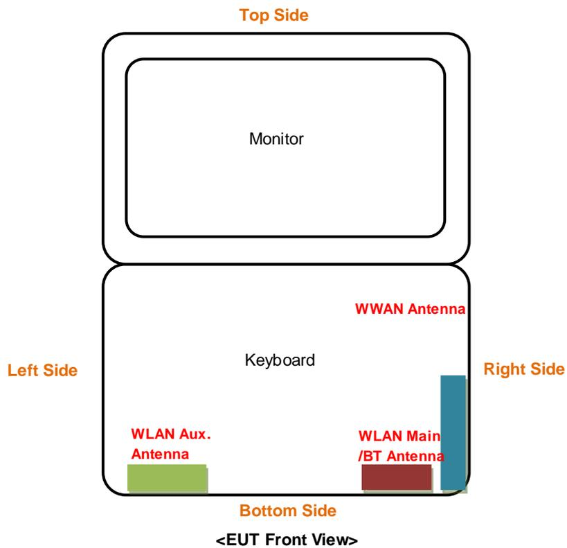
The separation distance for antenna to edge:
