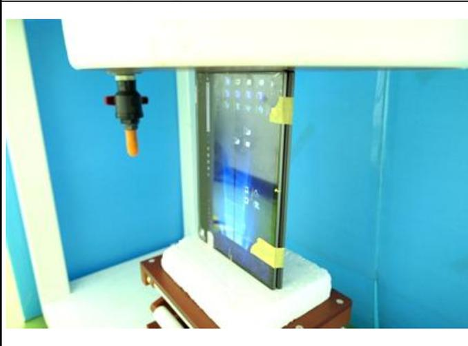
Body - Left Side of EUT at 0 mm
