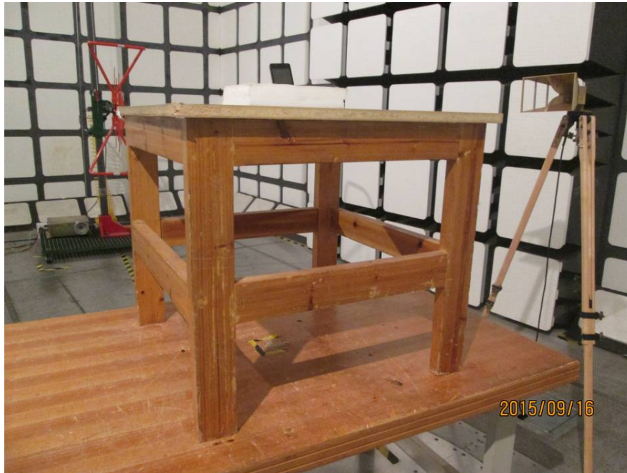
Radiated Emissions Test View (Below 1 GHz)
