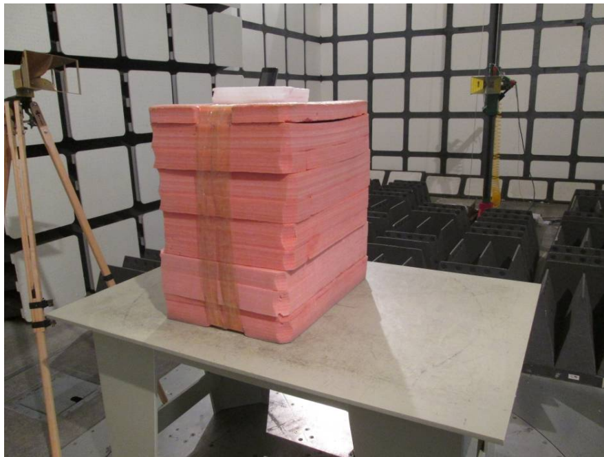
Radiated Emissions Test View (Above 1 GHz)
