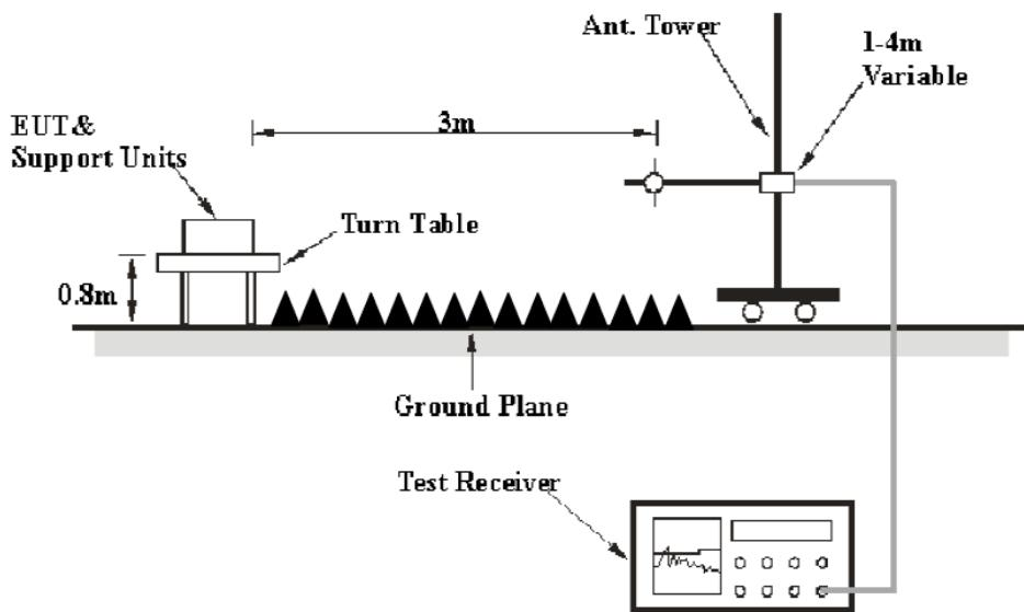
The radiated emission tests were performed in the 3 meters chamber test site, using the setup accordance with the ANSI C63.4-2014. The specification used was the FCC Part 15.109 Class B limits.
