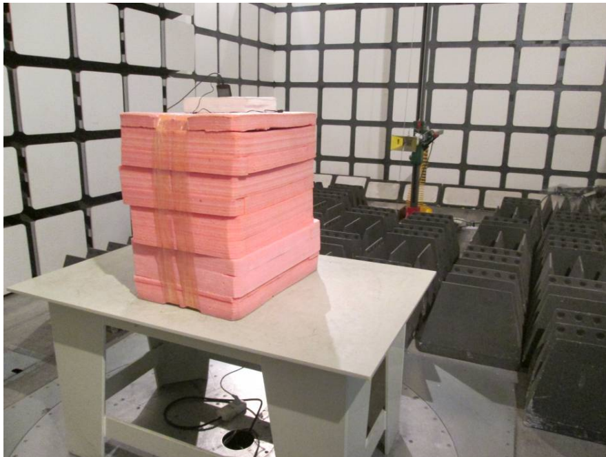
Radiated Emissions View (Above 1 GHz)
