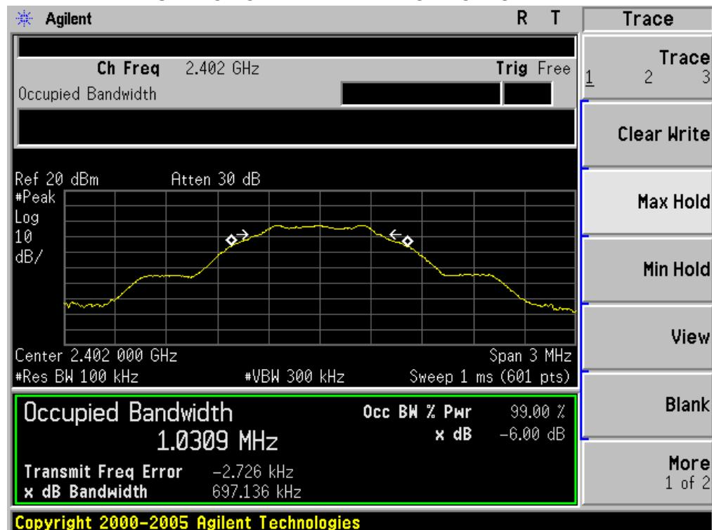
TEST PLOT OF BANDWIDTH FOR MIDDLE CHANNEL
