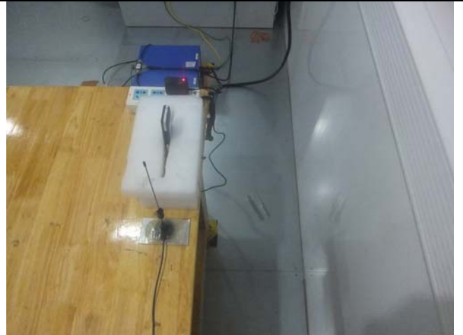
Conducted Emissions Test Setup Side View
