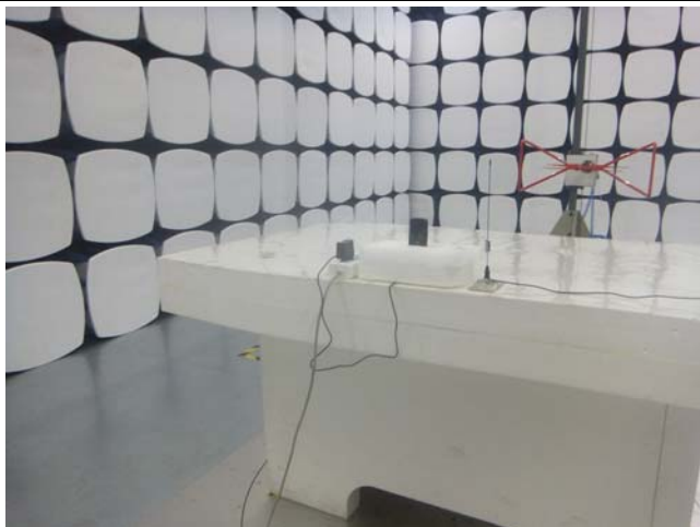
Conducted Emissions Test Setup Front View
