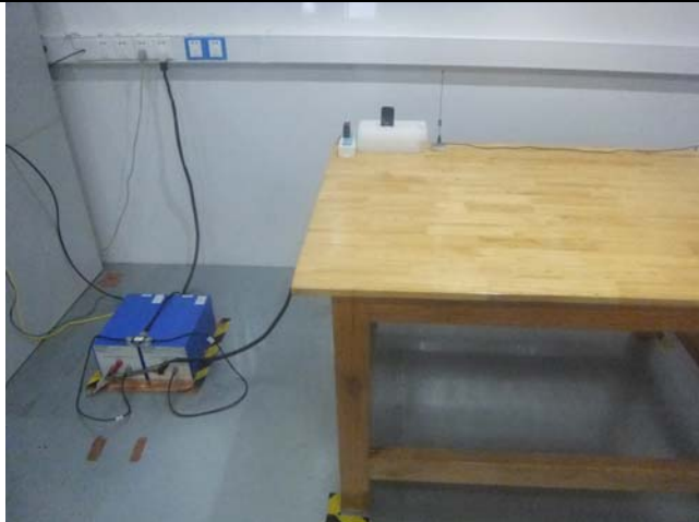
Conducted Emissions Test Setup Front View
