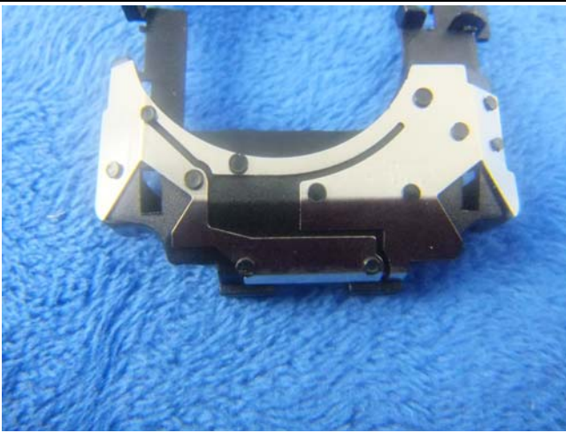
GSM Antenna View
