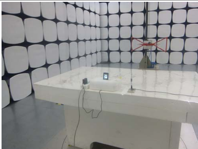
Radiated Spurious Emissions Test Setup Below 1GHz
