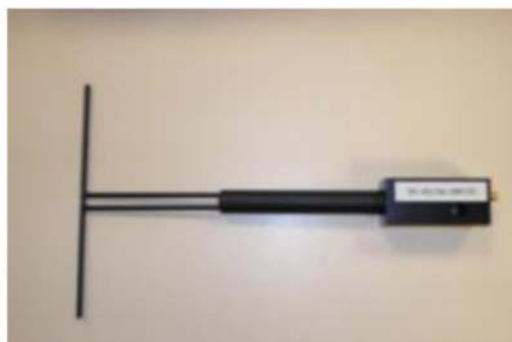
Figure 1 – Satimo COMOSAR Validation Dipole
