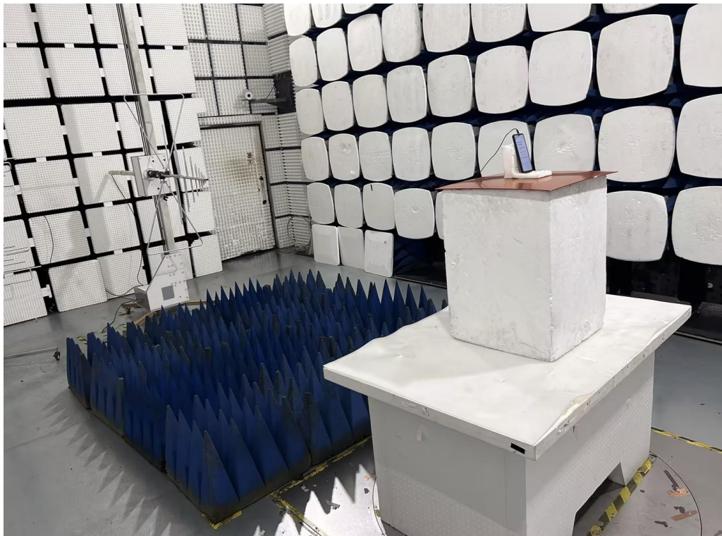
Radiated Emissions Measurement (Below 1GHz)
