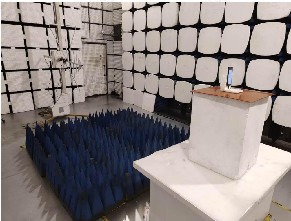
Radiated Emissions Measurement (Below 1GHz)
