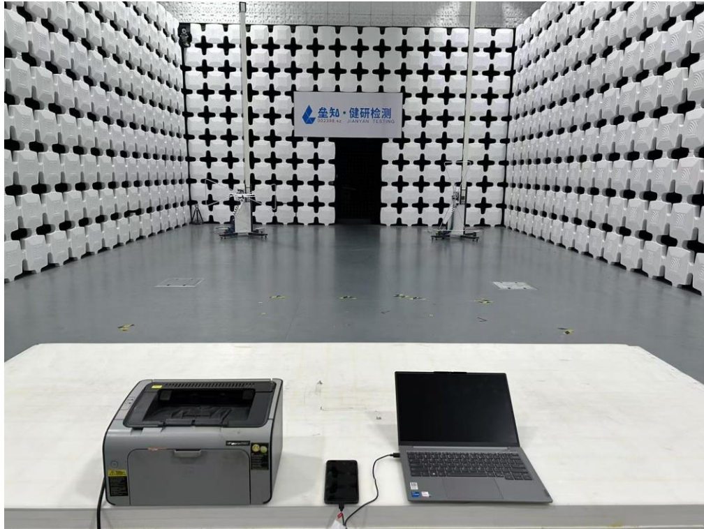
Radiated Spurious Emission Below 1GHz
