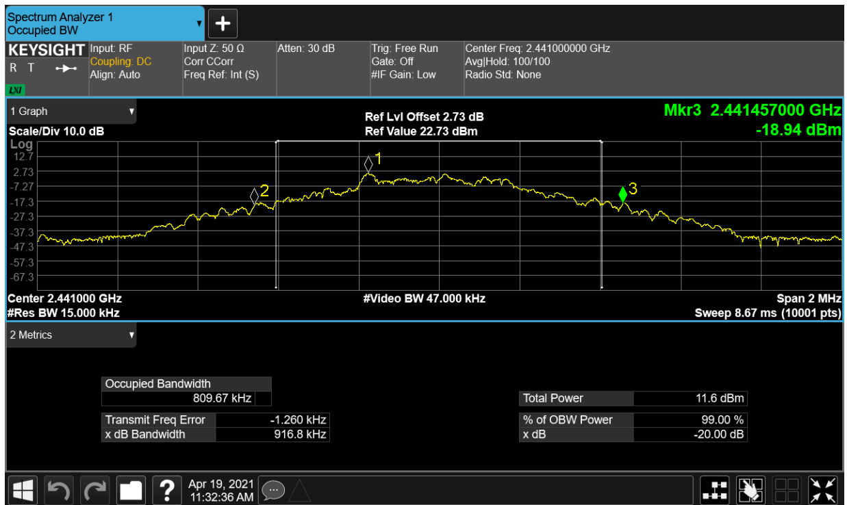
-20dB Bandwidth NVNT 1-DH1 2480MHz Ant1
