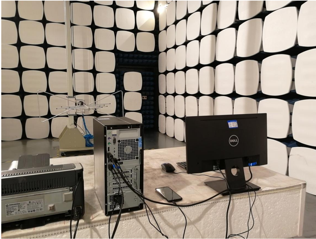
Radiated Emission Below 1GHz
