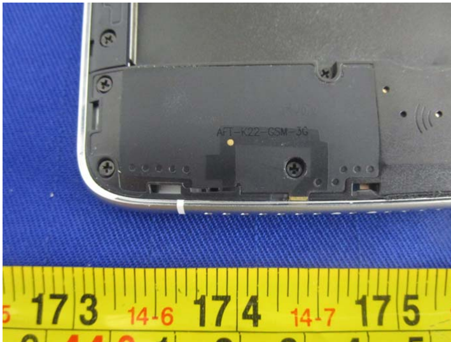
EUT –GSM&WCDMA Antenna View
