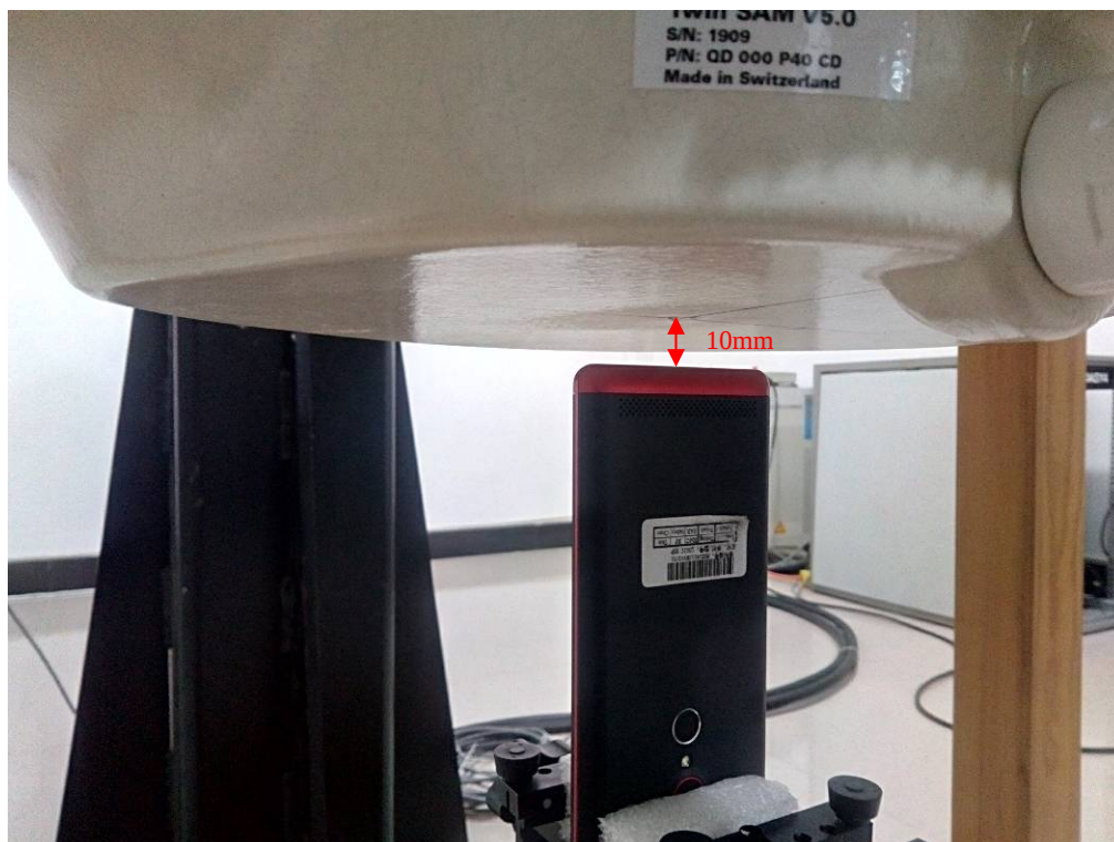
Body-worn Bottom Setup Photo (10mm)
