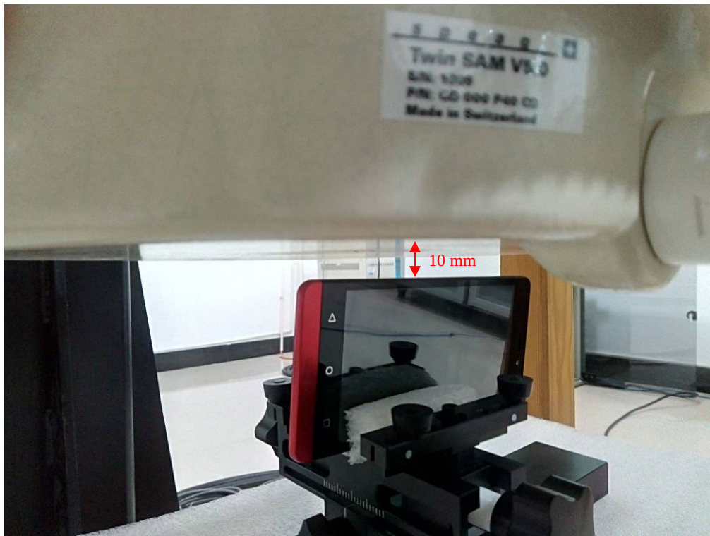
Body-worn Left Setup Photo (10mm)
