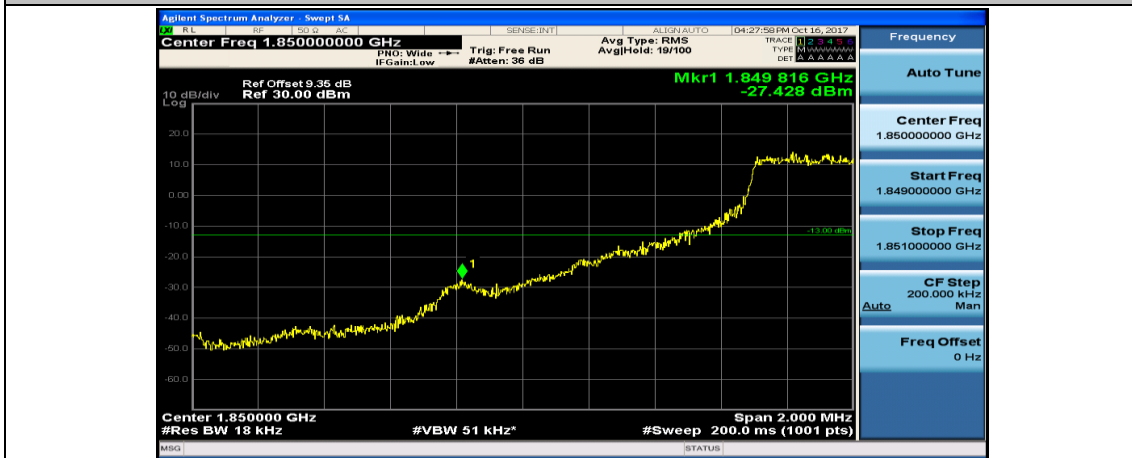
(Channel Bandwidth: 1.4 MHz)_LCH_16QAM_6RB#0
