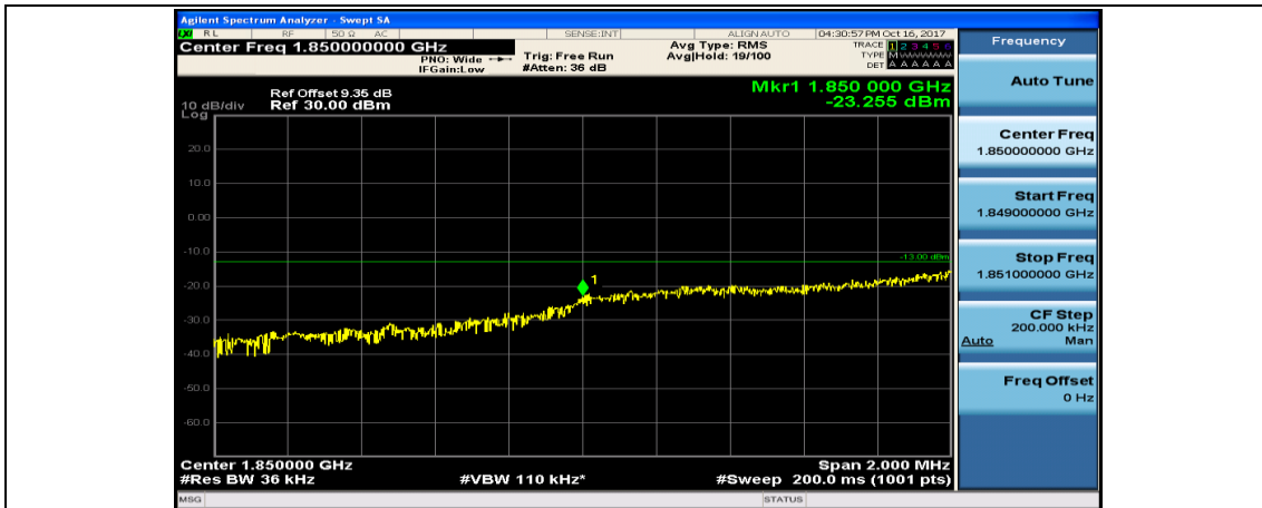
(Channel Bandwidth: 3 MHz)_LCH_QPSK_15RB#0
