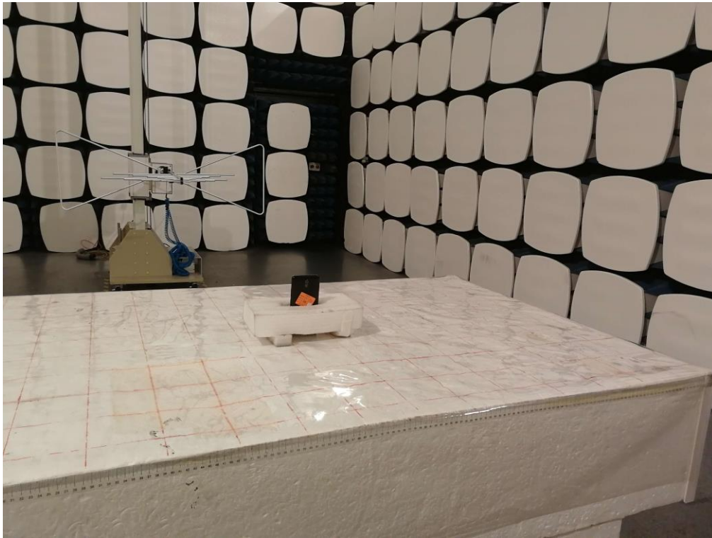
Radiated Spurious Emission Below 1GHz
