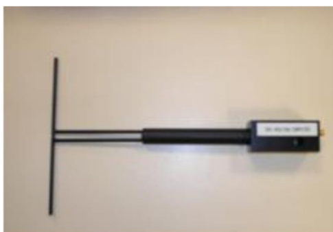
Figure 1 – Satimo COMOSAR Validation Dipole
