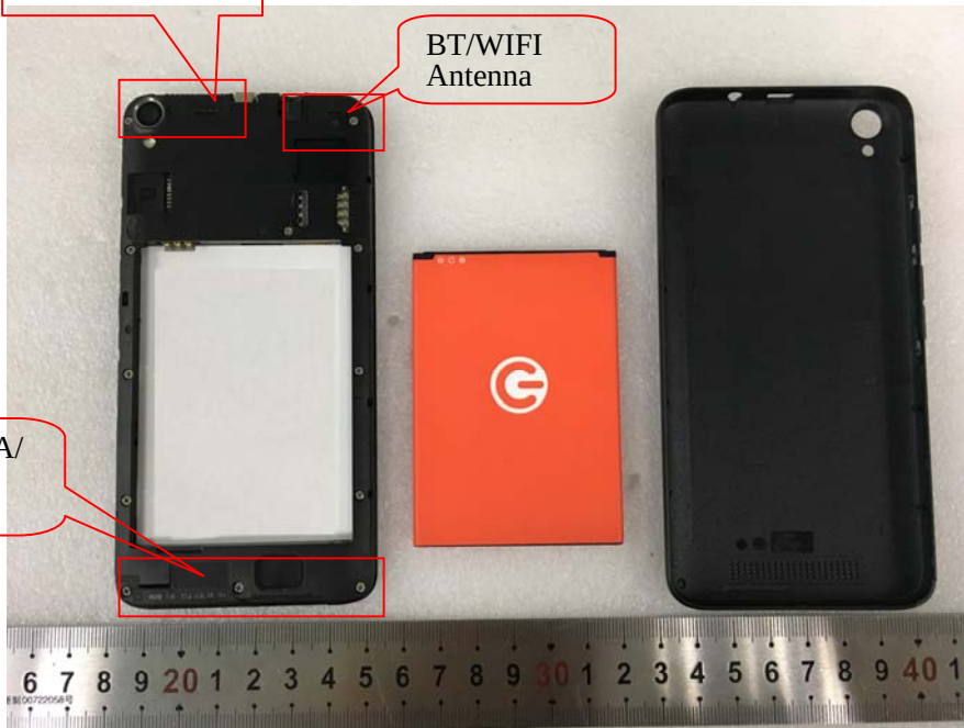
EUT – Cover off View 1
