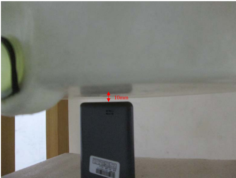
Body-worn Bottom Setup Photo (10mm)
