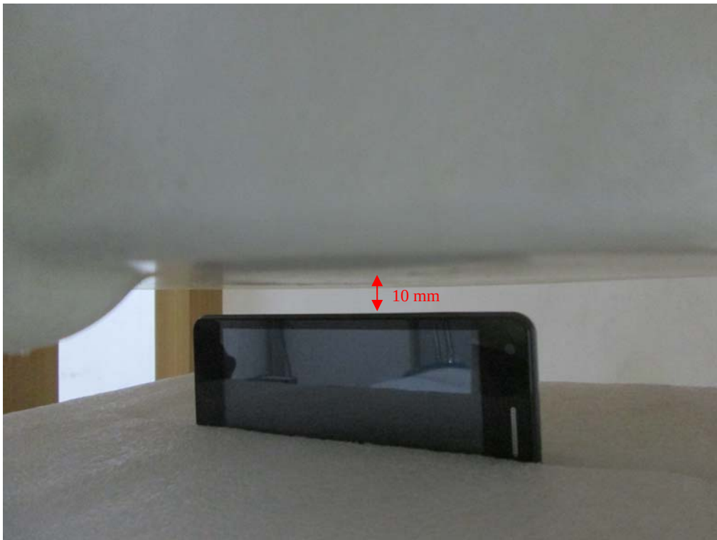
Body-worn Left Setup Photo (10mm)
