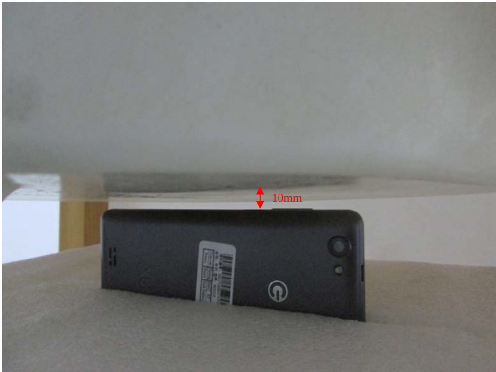
Body-worn Right Setup Photo (10mm)
