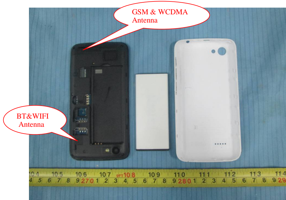
EUT –Cover off View 1
