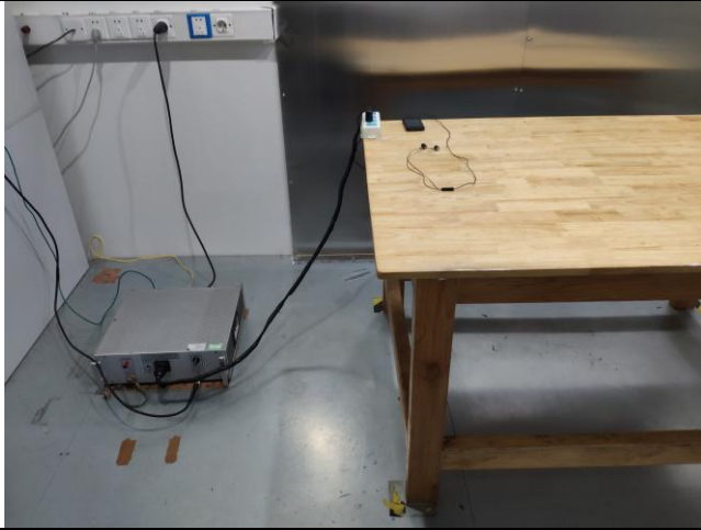
Conducted Emissions Test Setup Front View
