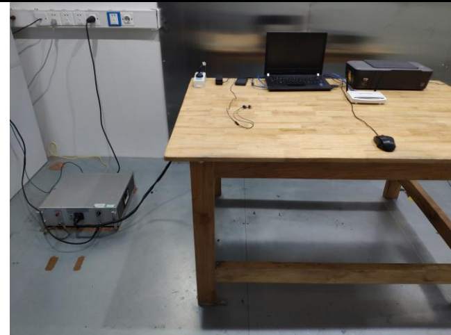
Conducted Emissions Test Setup – Front View
