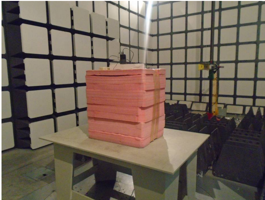
Radiated Emissions View (Above 1 GHz)
