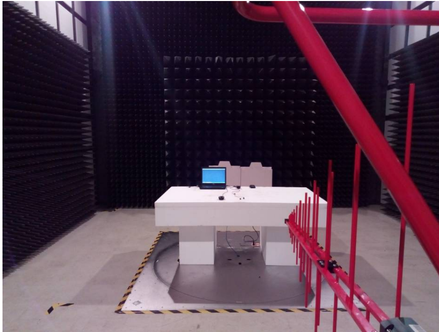
Radiated Emissions – Front View (Below 1 GHz)
