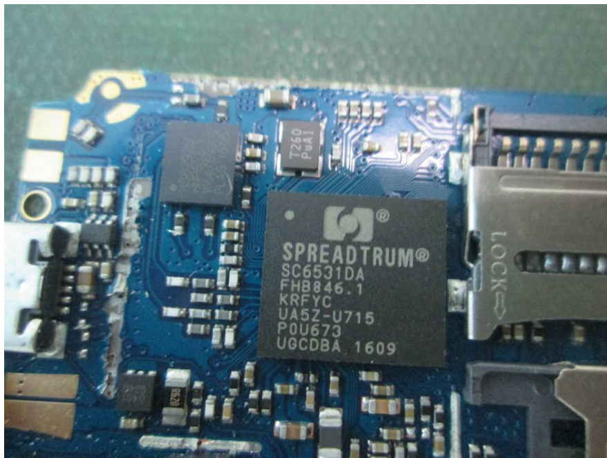
EUT –Main IC View
