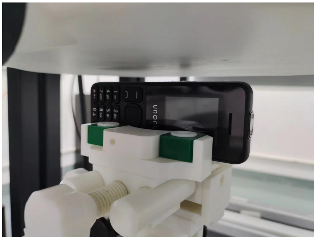
Body Left side (separation distance is 10mm)
