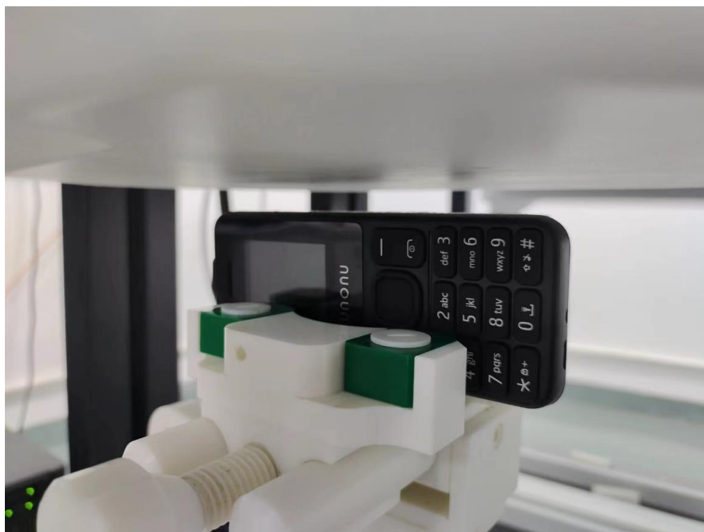
Body Right side (separation distance is 10mm)
