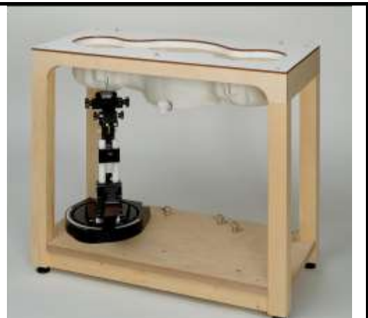
Fig. 8.7 Photo of SAM Twin Phantom
