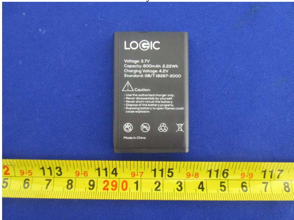
EUT – Battery Bottom View
