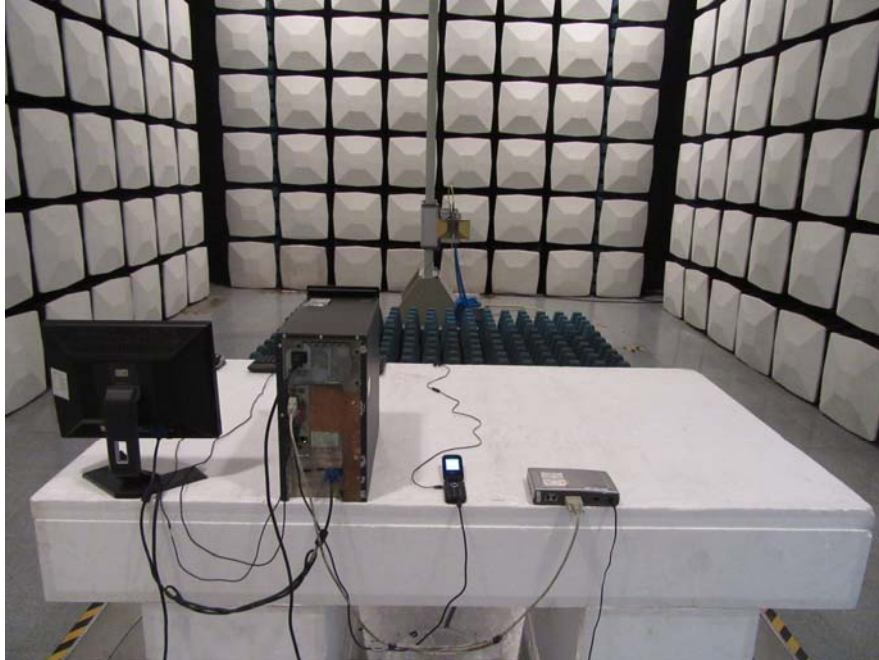
Radiated Emission - Rear View (Above 1 GHz)
