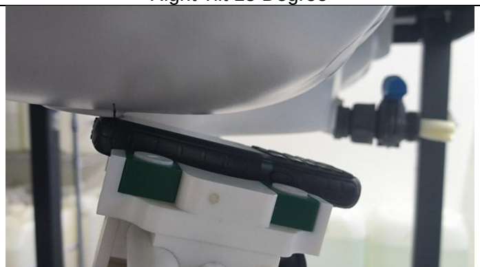
Back Side (Separation distance of 10mm)
