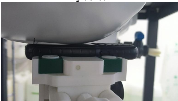
Front Side (Separation distance of 10mm)
