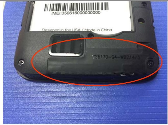
GSM/PCS/UMTS-FDD Antenna View
