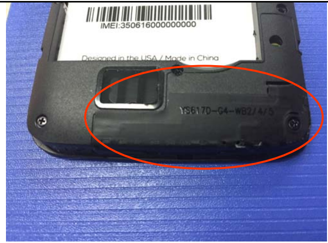
GSM/PCS/UMTS-FDD Antenna View
