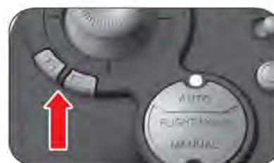
**IF DRONE SPINS COUNTER-CLOCKWISE** (VIEWED FROM ABOVE): Press the button several times until drone stops spinning.
