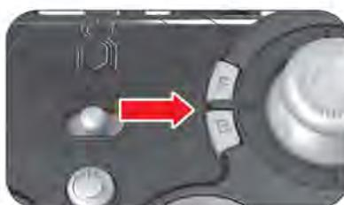
**IF DRONE DRIFTS FORWARD:** Press "B" button several times until drone stops drifting forward.
