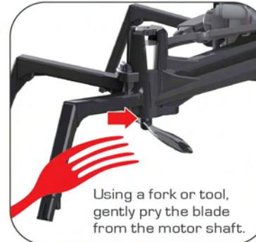
Using a fork or tool, gently pry the blade from the motor shaft.
