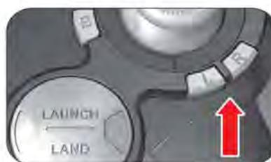
**IF DRONE DRIFTS LEFT:** Press "R" button several times until drone stops drifting left.
