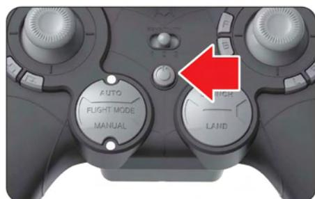
Turn on controller. [Before initial use, install new batteries into controller]
